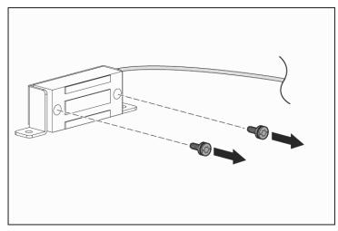
Remove the electromagnetic locks and cables from the rack.
