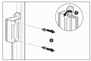
3. Remove the electromagnetic lock and cable from the rack
