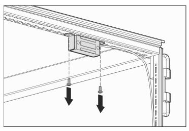
**3.** Using an Allen wrench, remove the two black cap screws securing each electromagnetic lock to its electromagnetic lock bracket.
