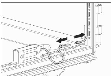
**NOTE:** Be sure to note the location of the electromagnetic brackets prior to removal.
