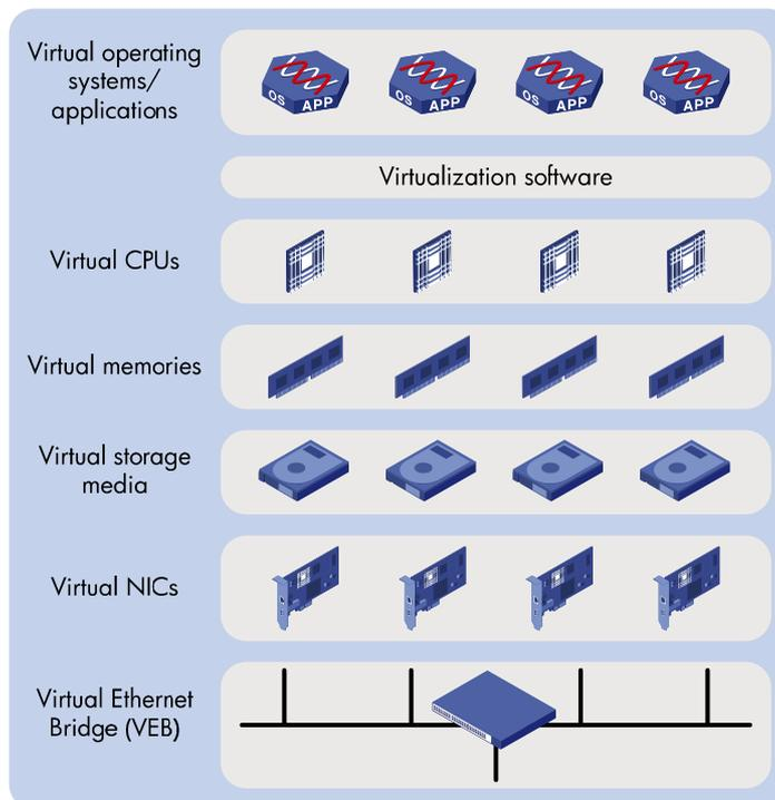
VMs on a physical server communicate with each other or with the outside network through a Virtual Ethernet Bridge (VEB). VEBs are implemented through software or hardware such as NICs. Both implementation methods have the following limitations:
