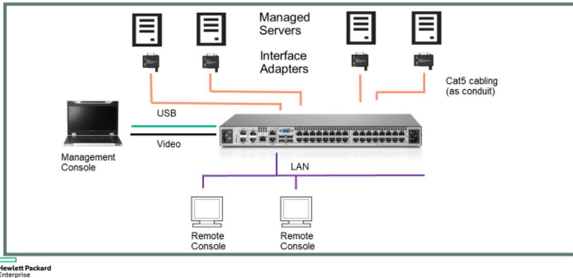
FIGURE 2. Digital (IP) KVM Switching
