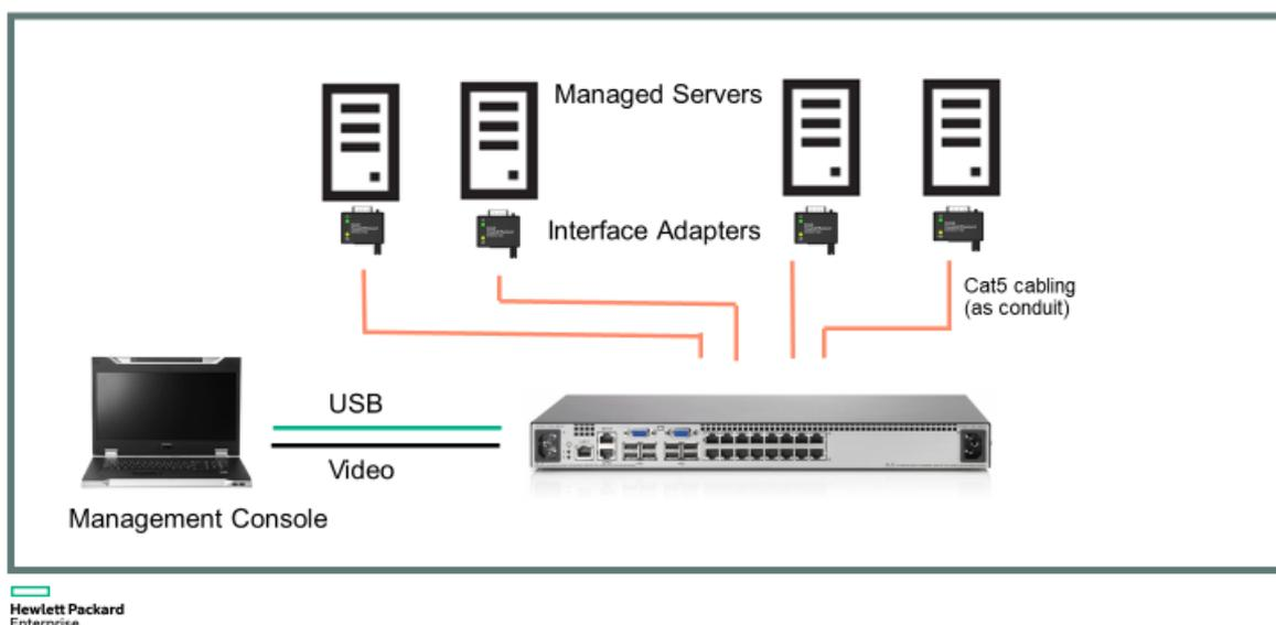
**FIGURE 1.** Analog KVM Switching
