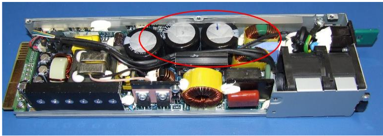
Electrolytic Capacitor (3 caps each in 4 PSU's)
