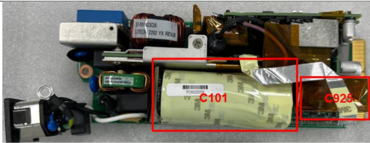
Attachment 10: Remove Electrolytic Capacitor (C103: 30mm*50 mm) from power supply HSTNS-PA67 .
