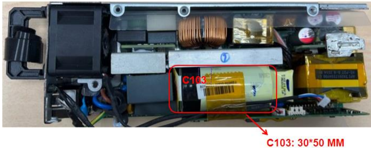
Attachment 10: Remove Electrolytic Capacitor (C103: 30mm*50 mm) from power supply HSTNS-PA67 .
