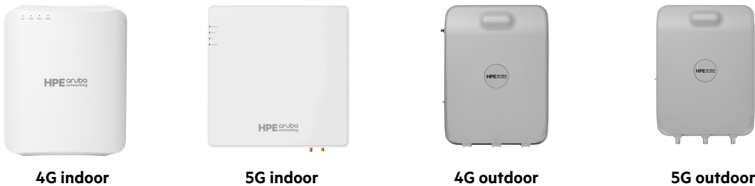
Figure 3. HPE Aruba Networking Small Cells. 4G options are available for enterprises in the US with 4G device ecosystems
