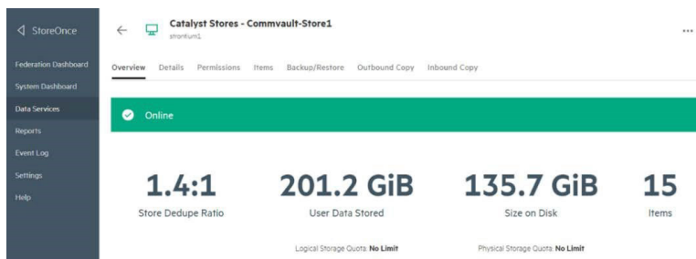
Figure 24. Overview of Catalyst Store after a first full backup of a 200 GB data set
