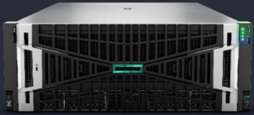
4U, 2P HPE ProLiant Compute DL380a Gen12 Ten NVIDIA RTX PRO™ 6000 or H200 NVL
