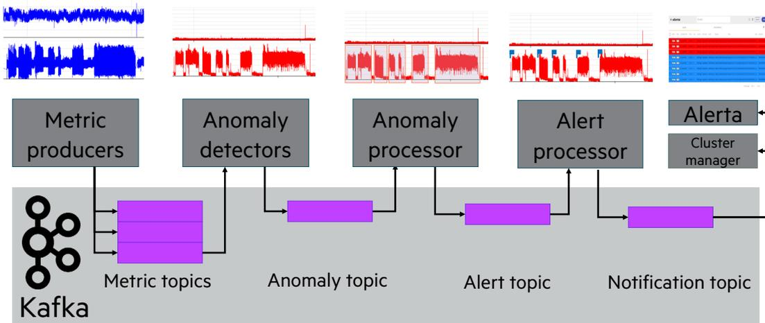
FIGURE 2. Anomaly detection workflow
