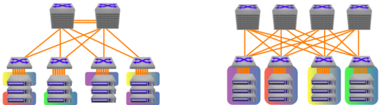
Arista Fixed System Leaf-Spine Designs Scale to 6,144 10GbE/25GbE ports or 1,536 40GbE/100GbE port at 3:1
