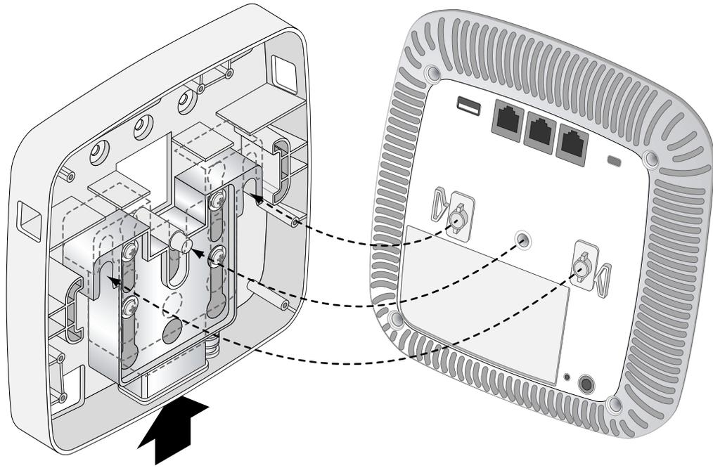
**Figure 6** *Completed Installation*
