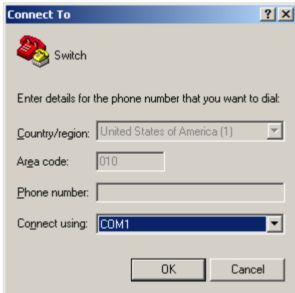
Figure 2 Set the serial port used by the HyperTerminal connection
