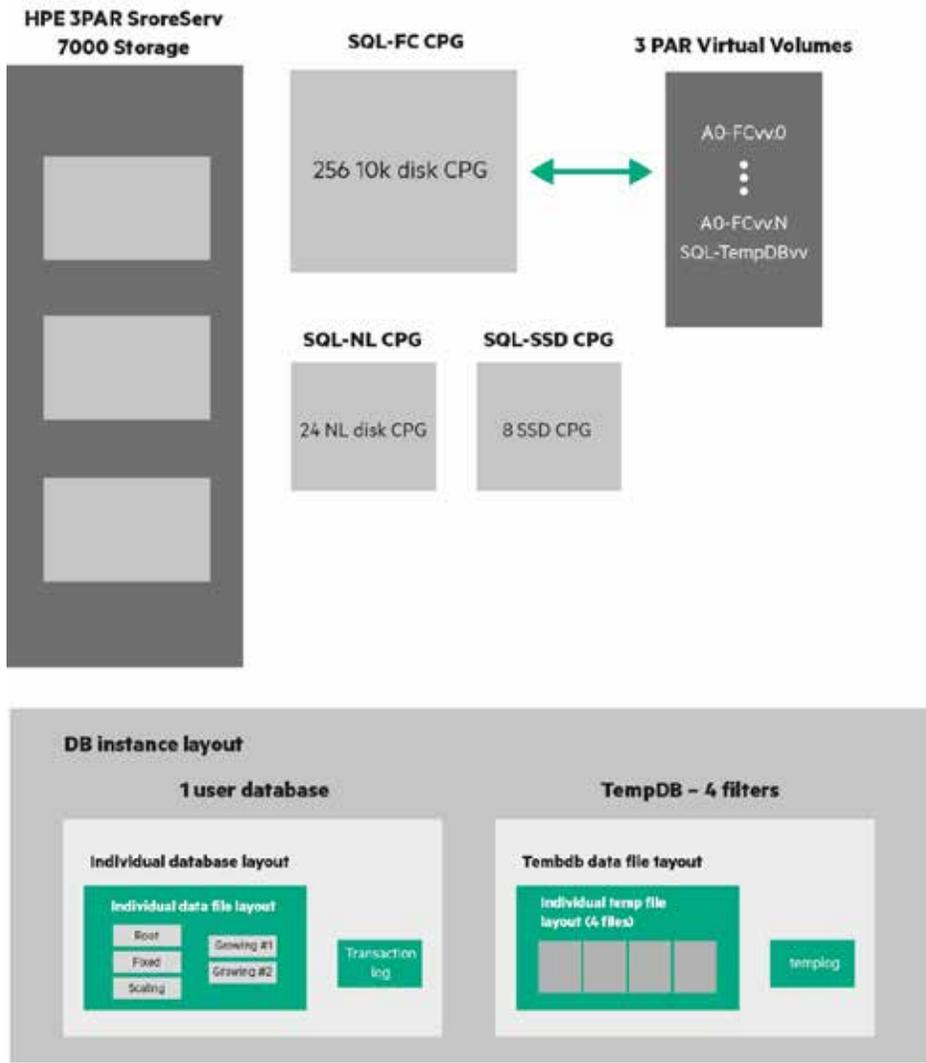
Figure 8. Typical DB instance layout created from HPE 3PAR Virtual Volumes
