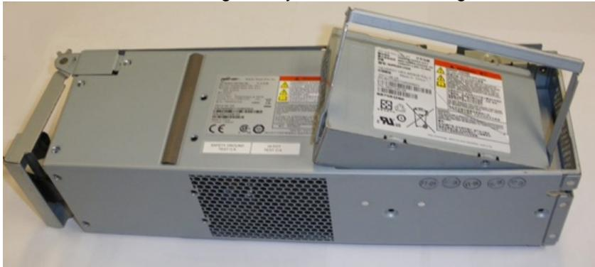
Remove the battery pack PCA from the enclosure
