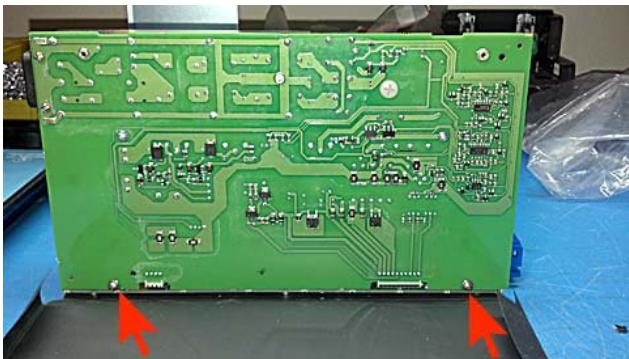
Slide the PCBA up and disconnect the Board wires
