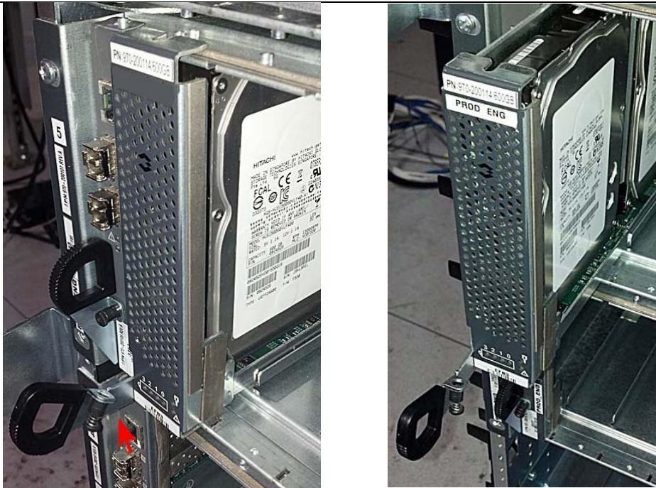
Remove screws holding each of the drive assemblies, and slide the HDD away from the connector to remove Hard Drive.
