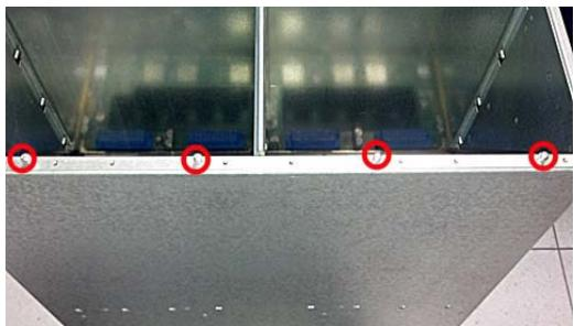
Pull out the cage assembly holding the PCBA from the main Chassis:
