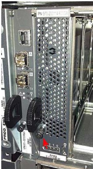
Pivot the handle downward and slide out the Dmag assy:
