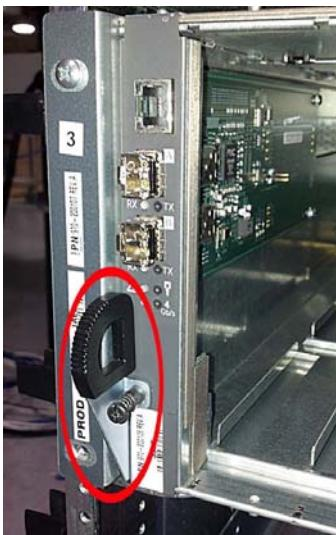
Remove screws holding the PCBA:
