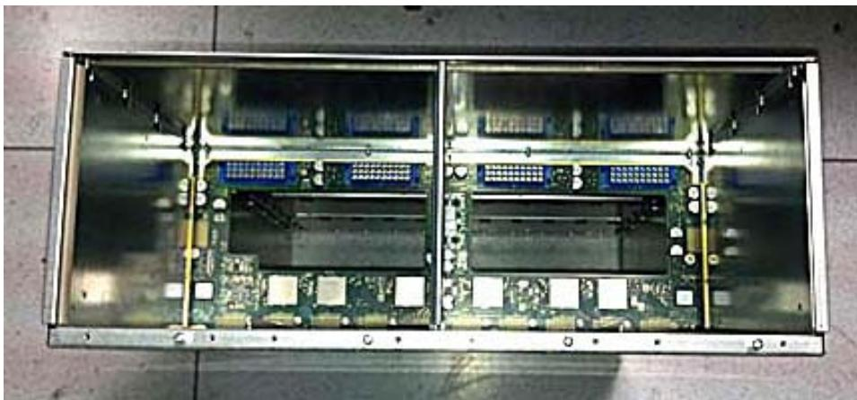
Remove the eight screws holding the Midplane PCBA:
