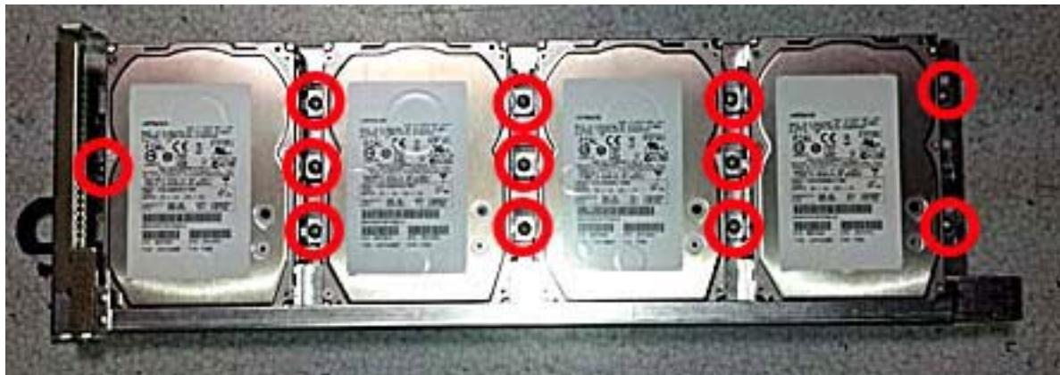
Remove the 9 screws holding the Sled PCBA and remove it.
