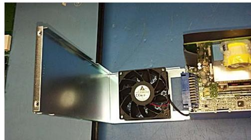
Disconnect fan connector to remove the cover w/ fan.
