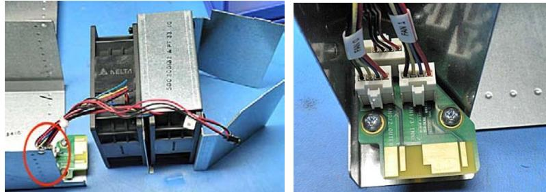
Remove three screws securing the PCBA.
