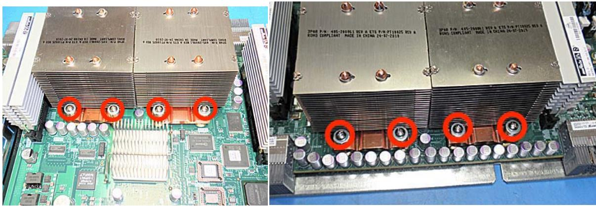
Remove the PCBA fastening screws to remove the PCBA.
