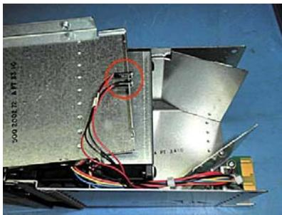
Remove Fan Assembly and disconnect all three fans at the PCBA.
