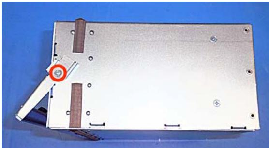
Remove screws securing the top cover.
