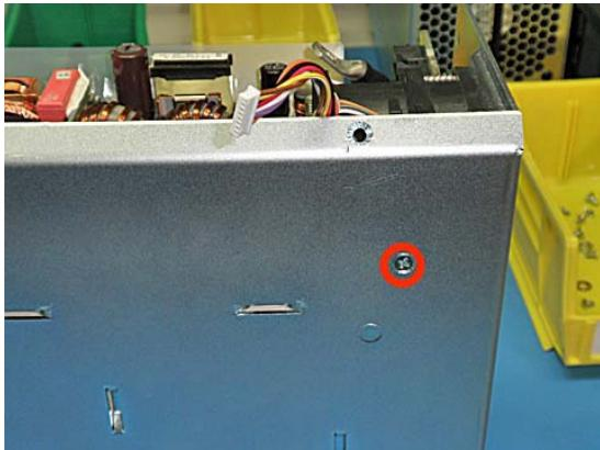
Remove the PCBA w/ Bracket Assy, and remove the PCBA screws.
