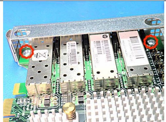
Remove the last PCBA screw at the back.
