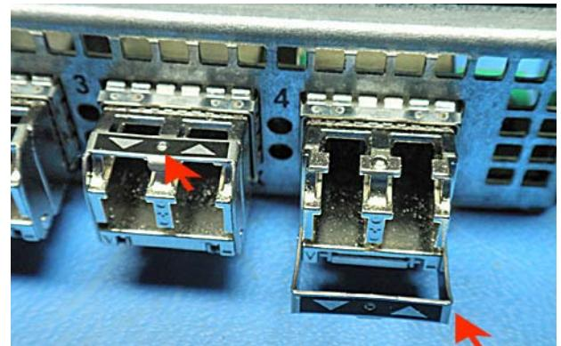
Remove the EMI gasket as shown.
