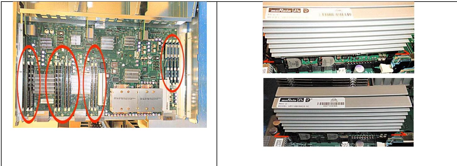
Remove the heat sink securing screws and remove the heat sinks.
