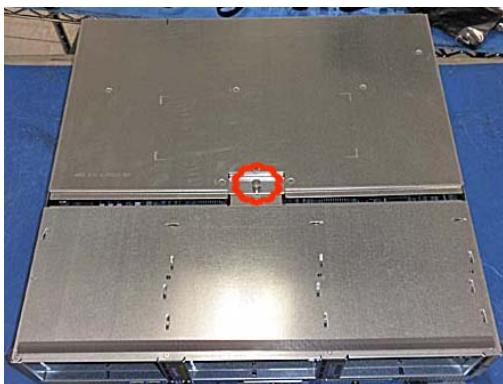
Remove side screws holding front Node Cover.
