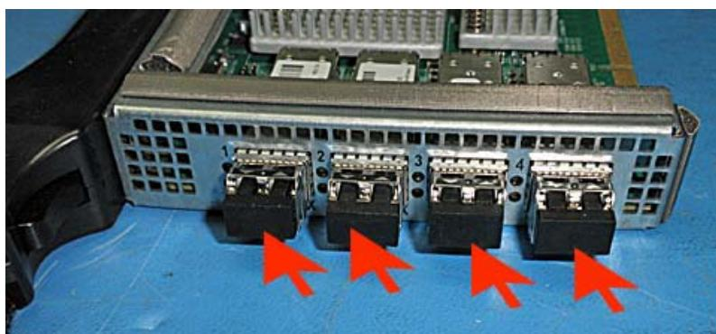
Lift and pull down at the same time on the SFP handle. Pull out the SFPs.
