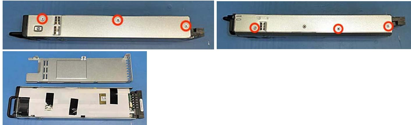
Remove four screws from the front side and one screw on the side. Disconnect connector to remove the fan.
