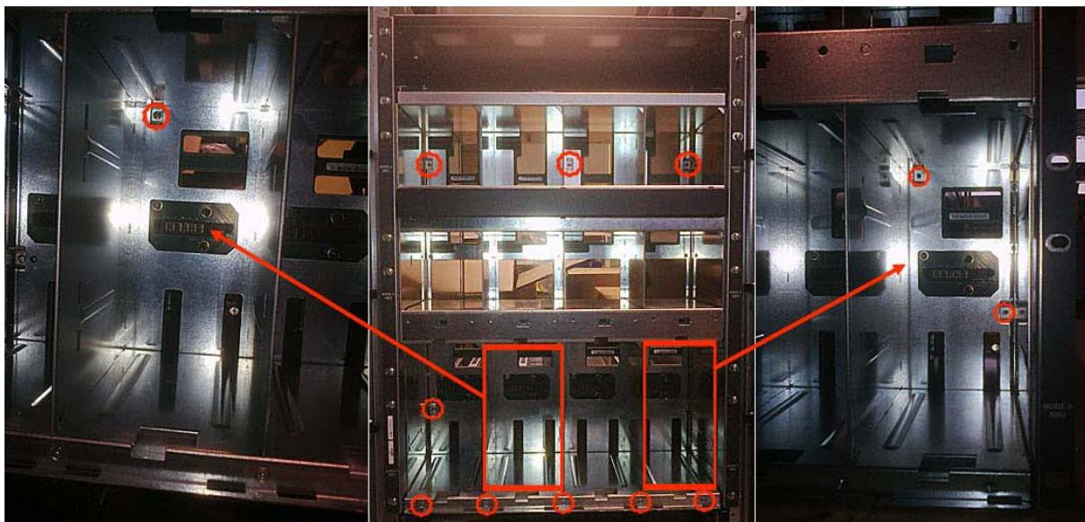
Pull out the Fan Module and BBU Cage.
