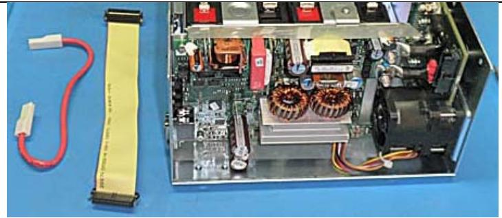
Disconnect power cables to the PCBA.
