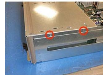
Remove the EMI gasket from the front, and remove six screws holding front Node Cover.
