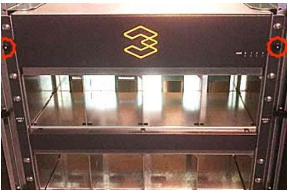
Pull out the Panel and remove the four screws securing the LED status board.
