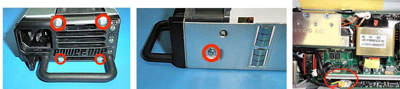
Remove six screws securing the main PCBA.
