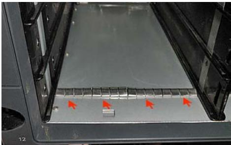
Remove one drive wall screw from each drive wall from the top, and one screw from each drive wall the bottom.
