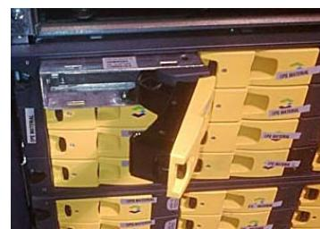
To remove hard drive: remove the 2 screws from the rear PCBA (if present) and remove the 4 screws from the bottom.
