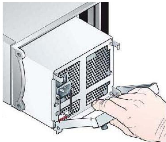
Use the following diagram for power supply disassembly:
