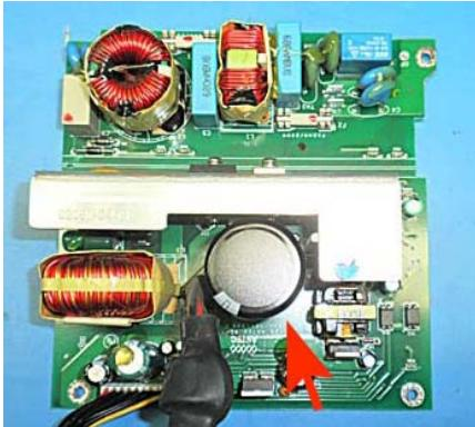
Remove the Connector PCBA
