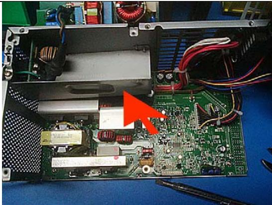
Remove the large capacitor from the Small PCBA.
