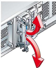
Grip the latch handles and withdraw the module.
