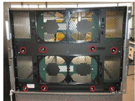
Remove all the 7 top screws and 8 screws on each side.
