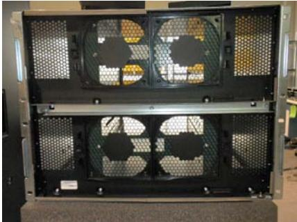
Remove the center rail, 3 nuts.
