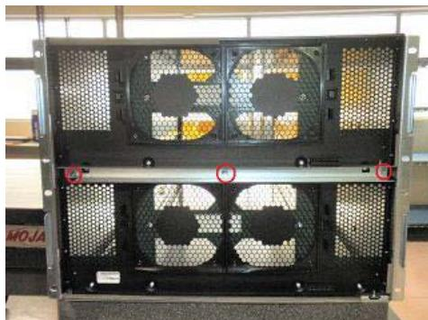
Remove the front shroud screws, 8x.
