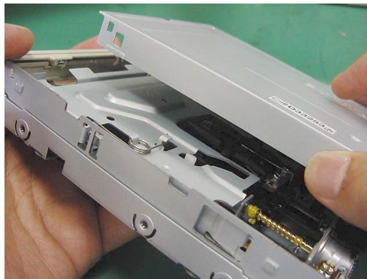
Figure 10. Removing the shield cover from the FDD
