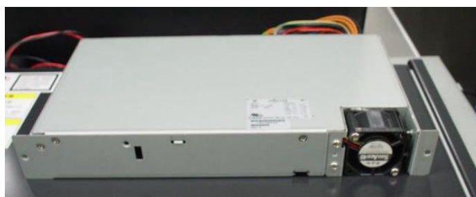
Figure 16. Removing the power supply HS0102
