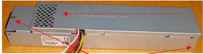
2 x crosshead screws, to remove the lid from the PSU
