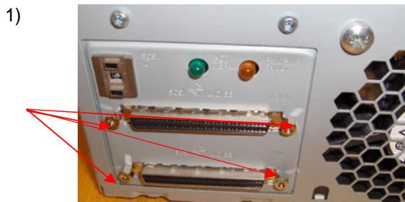
Remove 4 x securing nuts to remove the I/O SCSI PCA
