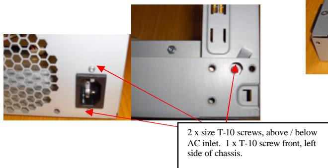
2 x size T-10 screws, above / below AC inlet. 1 x T-10 screw front, left side of chassis.
