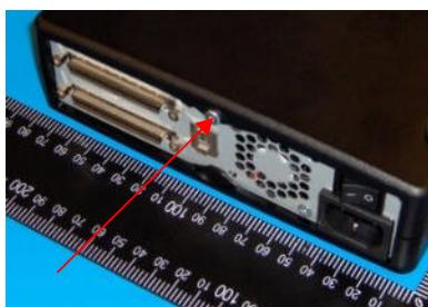
1) Remove 1 x T-8 screw from rear of lid / chassis. Use a flathead screwdriver to unclip the catches securing the lid to the chassis.
