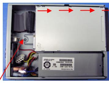
2) 1 x T-15 screw to remove the mechanism. Mechanism & base plate will then slide out in direction of arrows.
