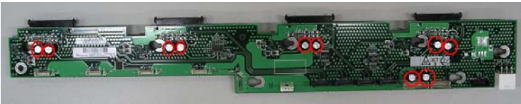
Item 1: Remove screw from PCB
