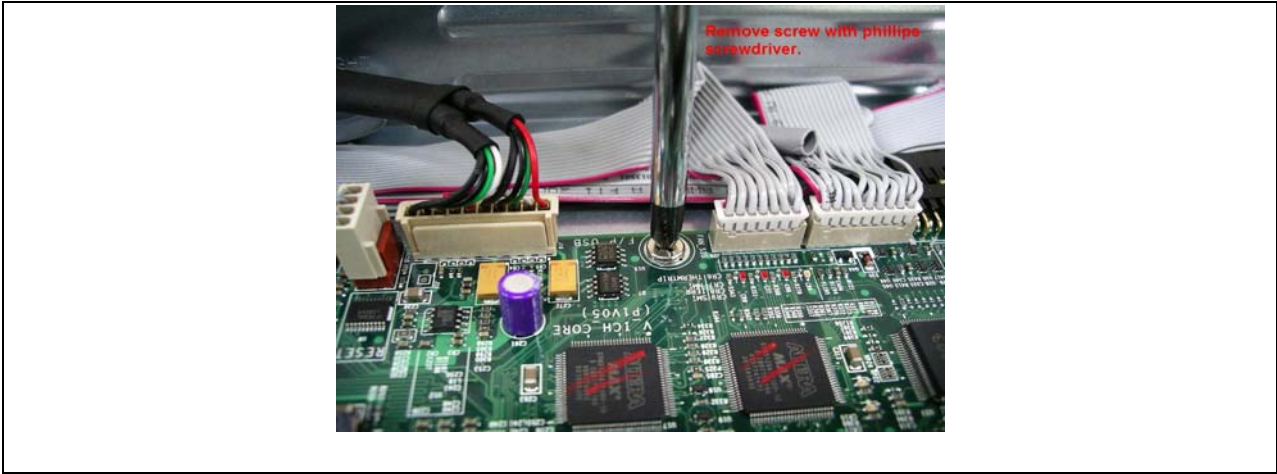
Item 1: Remove screw from PCB
