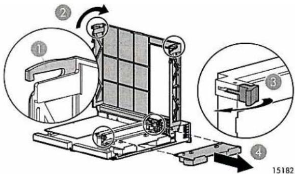
1. Push down on the battery retaining clip, located near the lower corner of the module.
