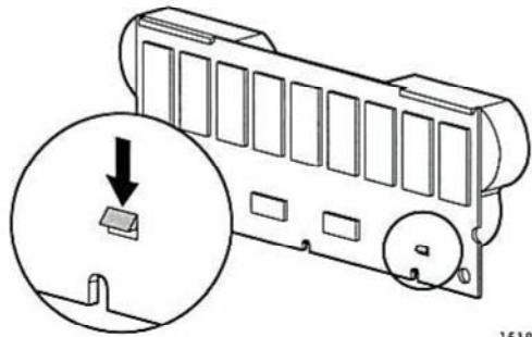
2. Swing the battery pack away from the module to a 30-degree angle, and then lift the battery pack upward to unhook the top of it.
