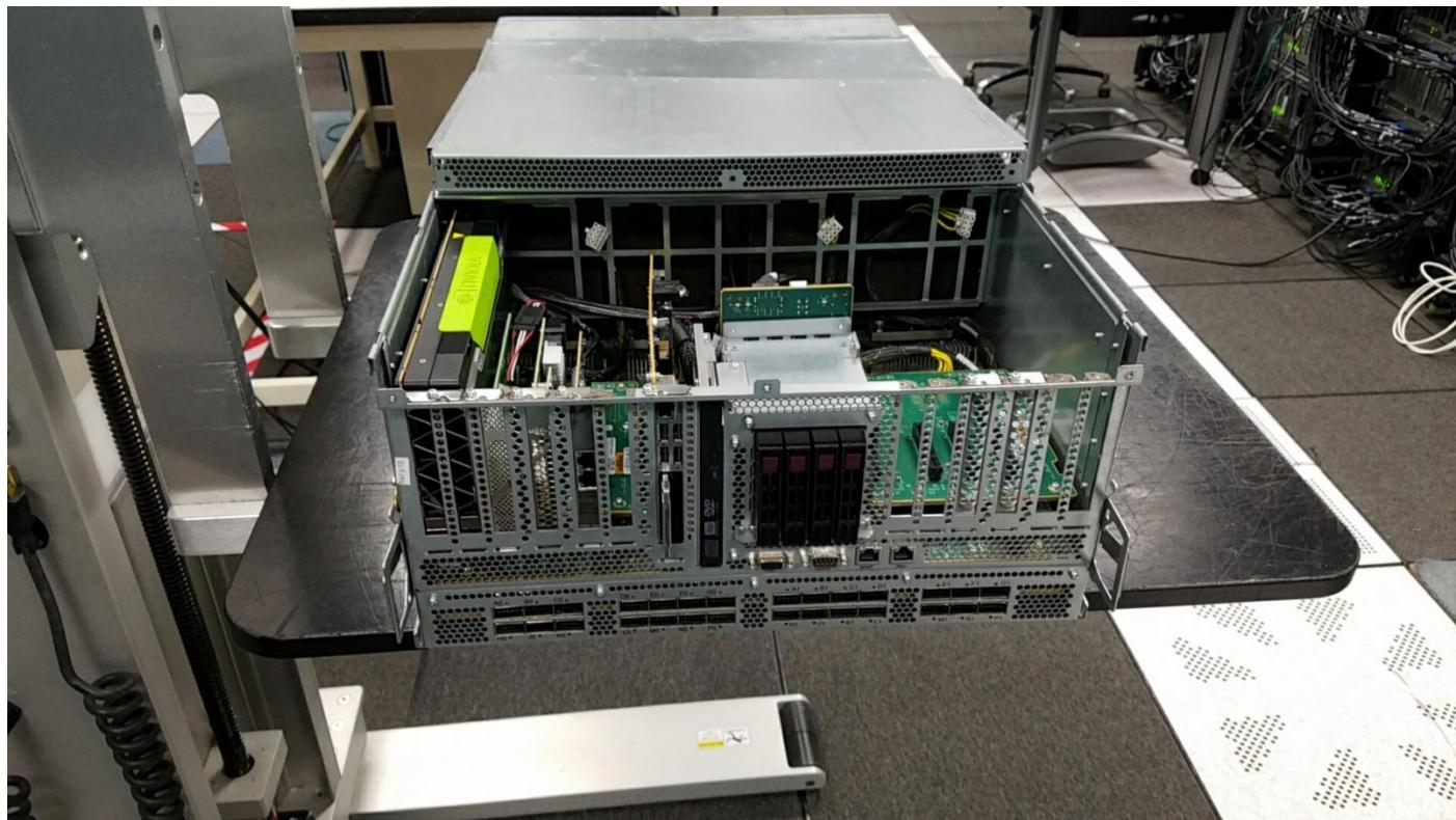
Then remove coin cell A and supercap by removing PCI faceplate P1 retention screw C and then remove supercap B.
