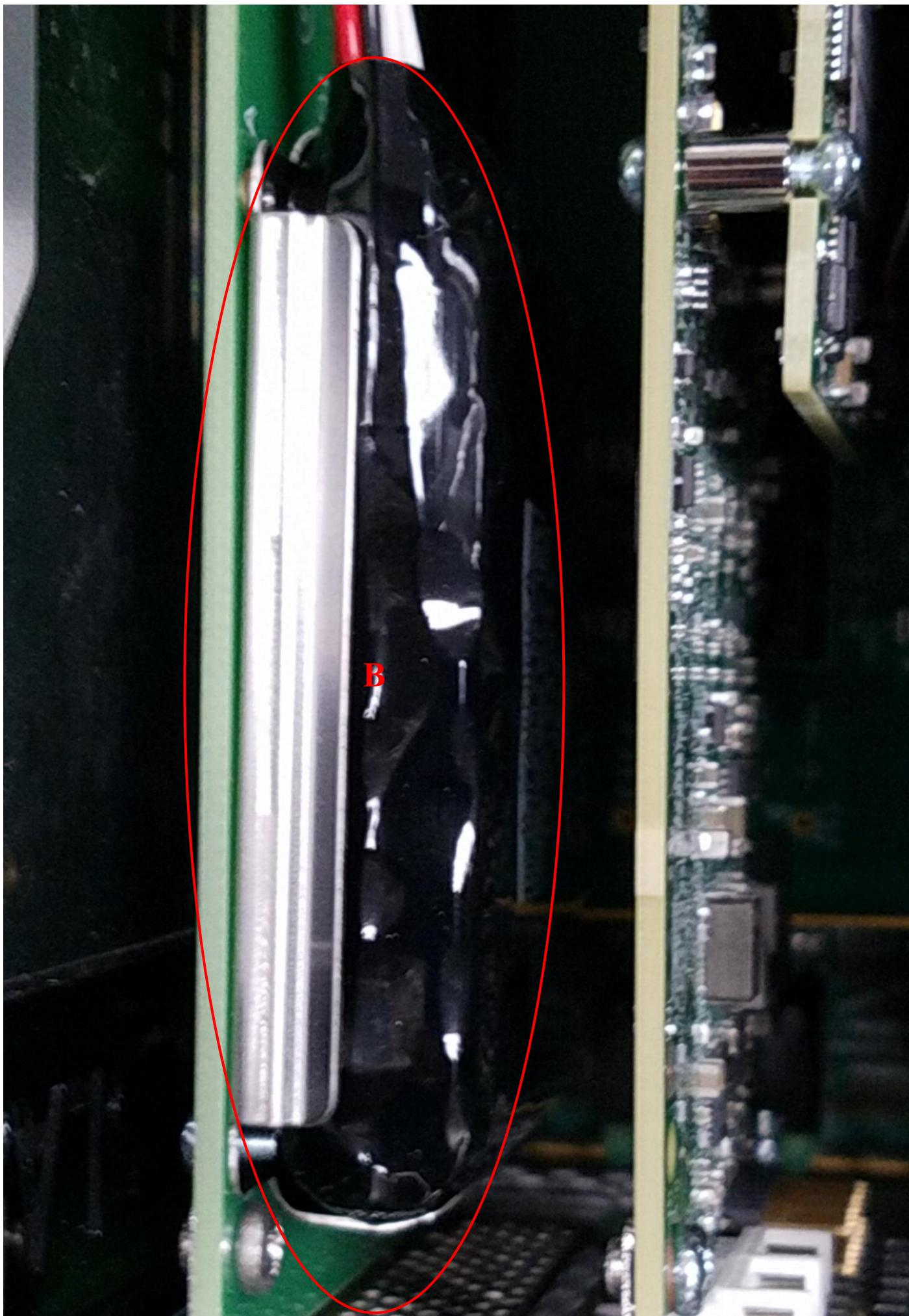
Power Supply capacitor removal.
