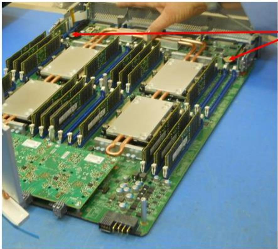
Batteries to be removed (2 for each **Serverboard** at most)
