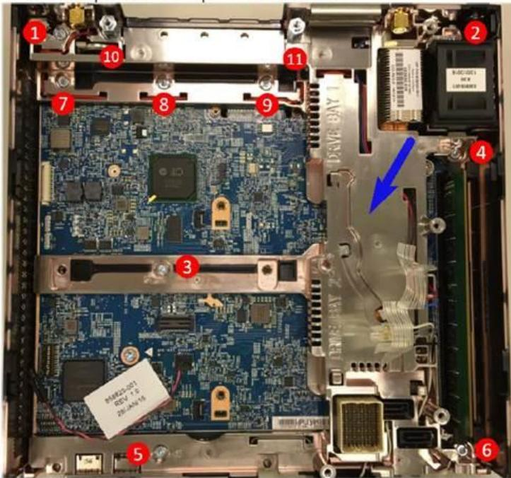
Attachment 4- Plastic with metal coating- Blue Arrow. Dispose of properly
