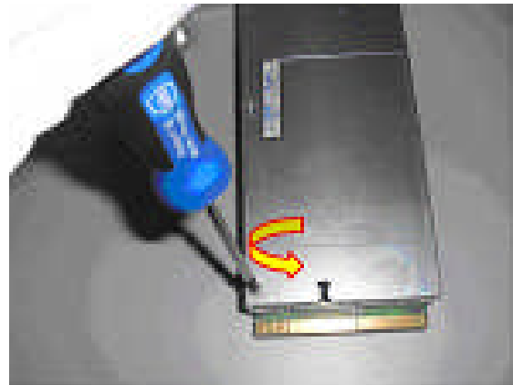
Figure 20 Remove the screws of the inside PSU
