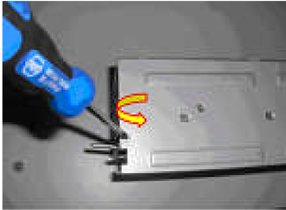
Figure 17 Remove the top screws of the PSU
