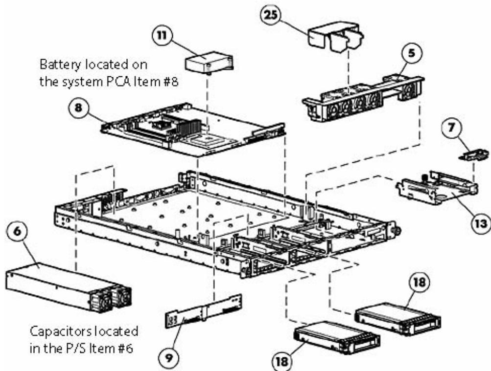
Printed circuit boards or printed circuit assemblies: Item 6, 8, and 9
