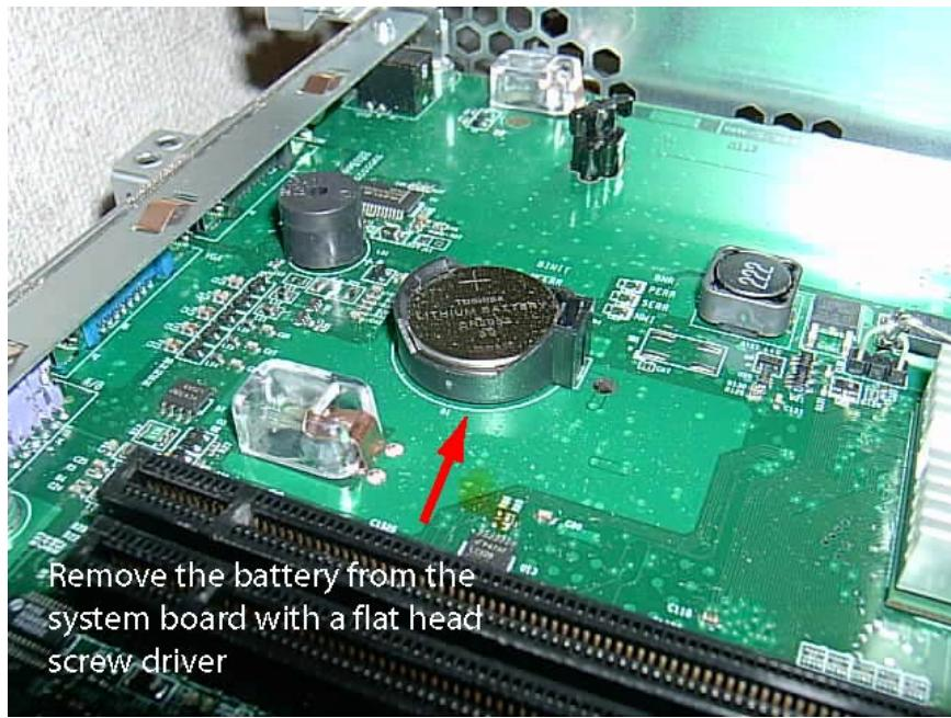
Remove the battery from the system board with a flat head screw driver
