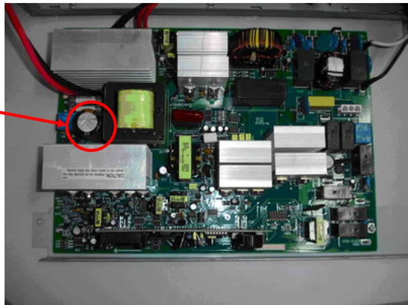
The PSDR PCB assembly of High Voltage unit
