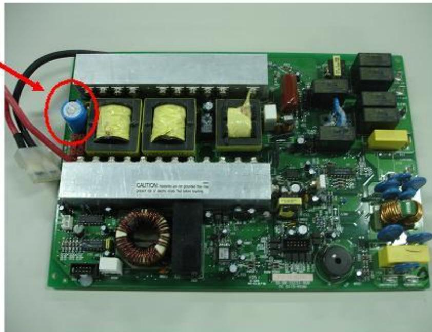
The PSDR PCB assembly of Low Voltage (US/TWN/JPN) unit
