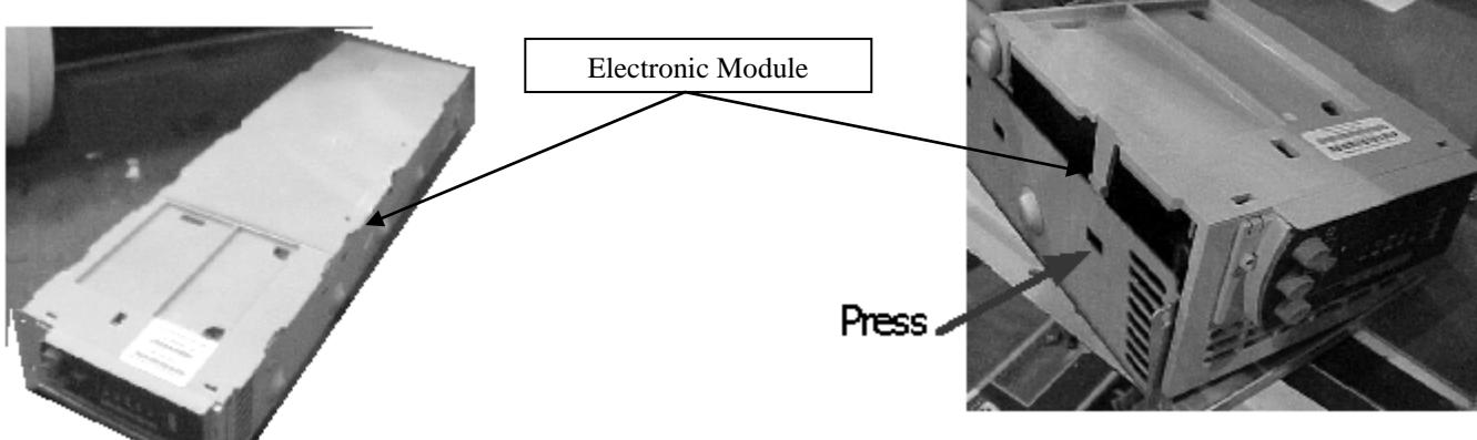
**Remove X-Slot and electronic module board with a Philips screwdriver.**
