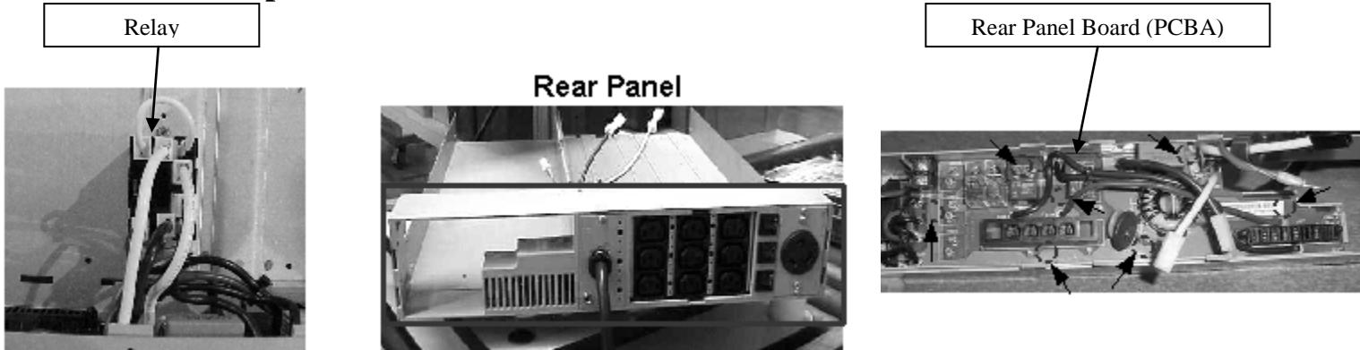
**3.2.2 Disassemble of the Electronic module: Pry snaps to remove cover, front and rear panel from the module.**
