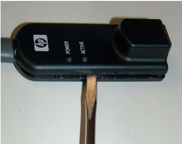
Prying Top and Bottom Cover with Screw driver
