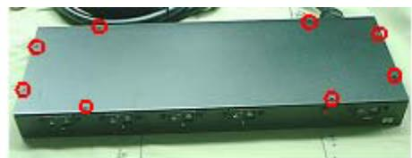
Disassemble the case base screws with screwdriver.
