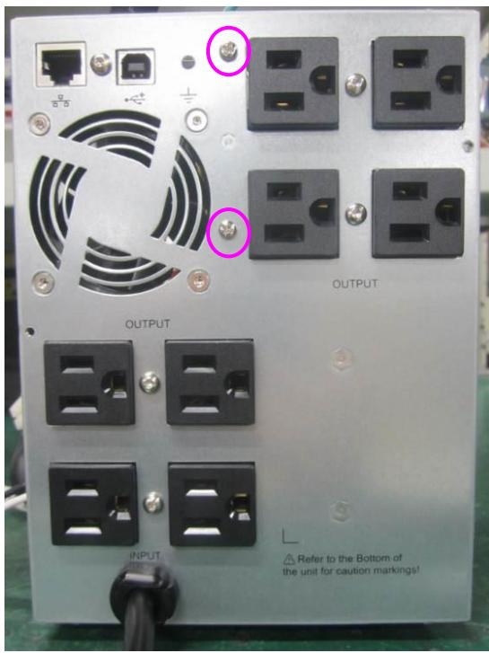
Step 6: Remove screws as below picture, uninstall inlets, Fan, USB & PCBA.
