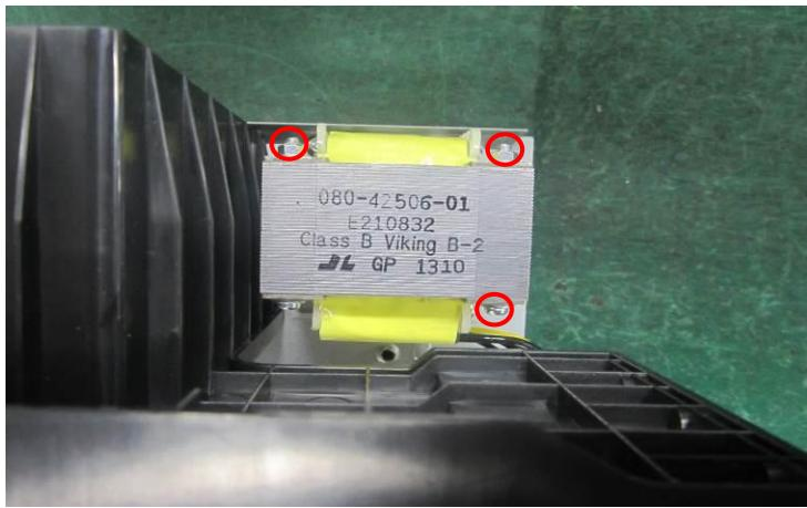
Step 9: Remove screws from bottom and front side, uninstall the plastic battery bracket.
