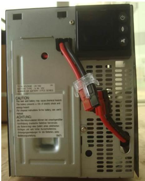
Step 4: Uninstall battery metal cover by removing screw as below, take out battery
