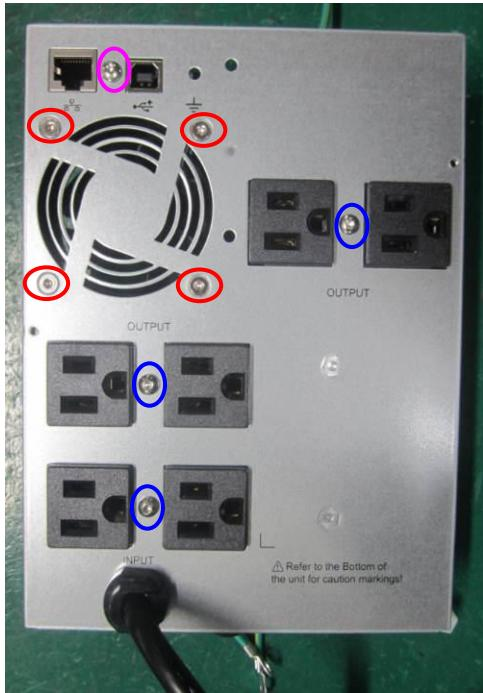
Step 7: Disconnect wires, remove screws as shown below, take off main PCBA.
