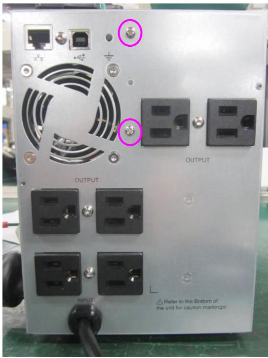
Step 6: Remove screws as shown in below picture, uninstall inlets, Fan, USB PCBA.
