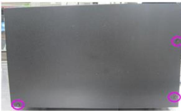
Step 3: uninstall LCD BOX manually, disconnect the flat wire, and then take off 2pcs screws by screw driver, remove LCD from LCD BOX.
