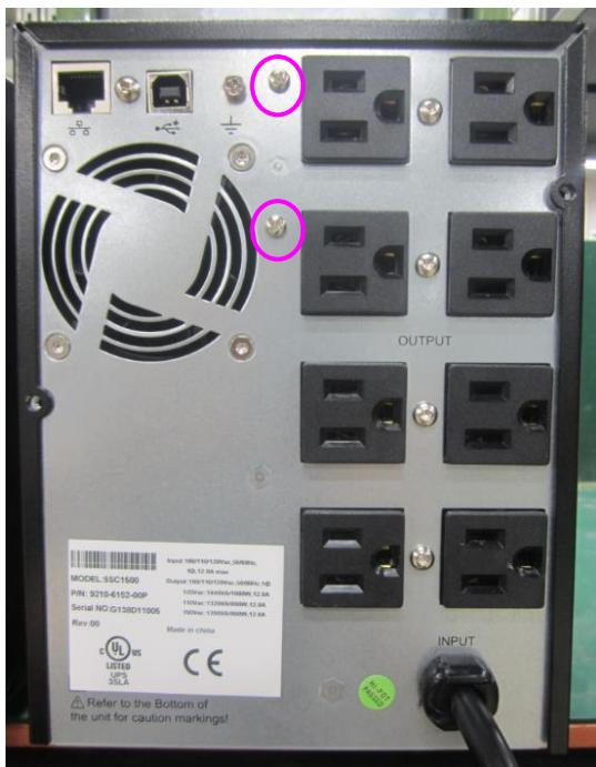
Step 6: Remove screws per below picture, uninstall inlets, Fan, USB & PCBA.
