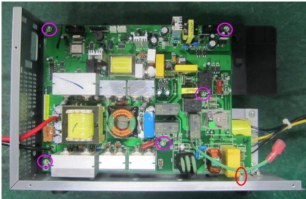
Step 8: Remove screws and uninstall TX.
