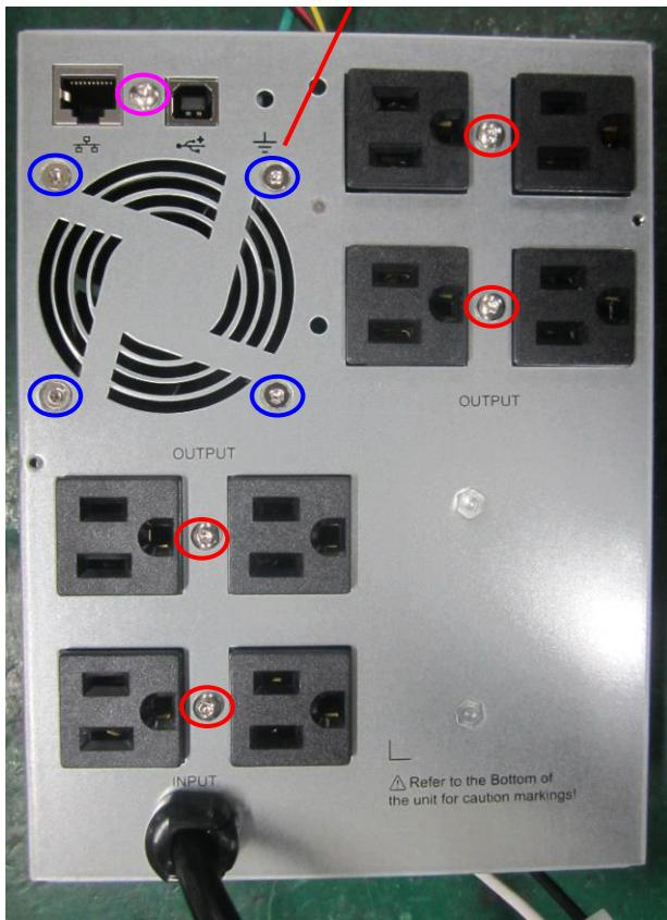
Step 7: Disconnect wires, remove screws as below shown & take off main PCBA.
