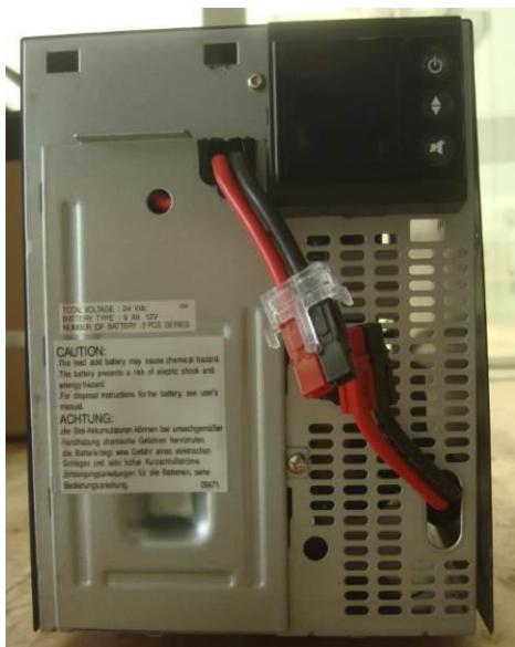
Step 4: Uninstall battery metal cover by removing screw as below, take out battery pack.
