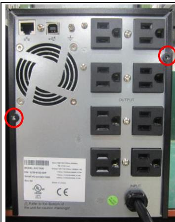
Step 3: uninstall LCD BOX manually, disconnect the flat wire, and then take off 2pcs screws by screw driver, remove LCD from LCD BOX.
