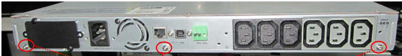
10. Remove the RPO connector, loosen the screws fixing Slot box, COM PCBA, and rear FAN, loosen the nut fixing ground cable and then remove the Slot box, COM PCBA, and rear FAN, outlet.
