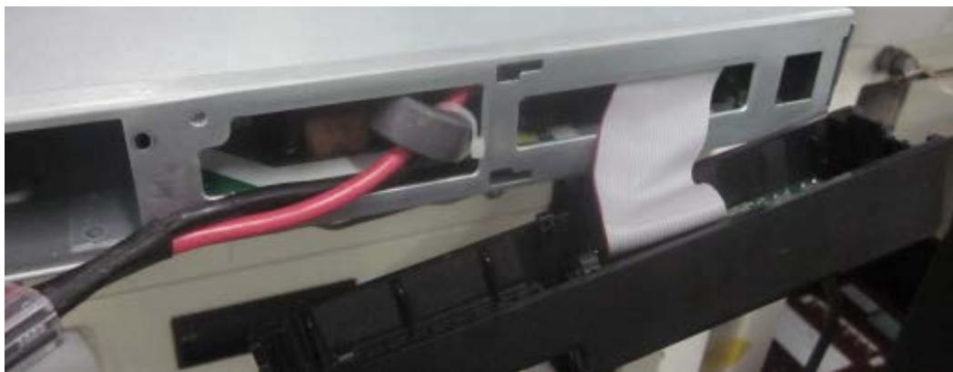
5. Disconnect the LCD cable and PCBA.
