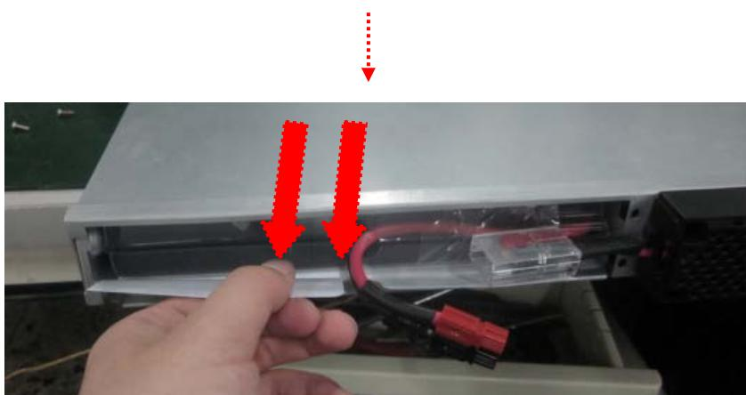
4. Loosen the screws fixing the right panel ASSY, and remove the right panel ASSY.
