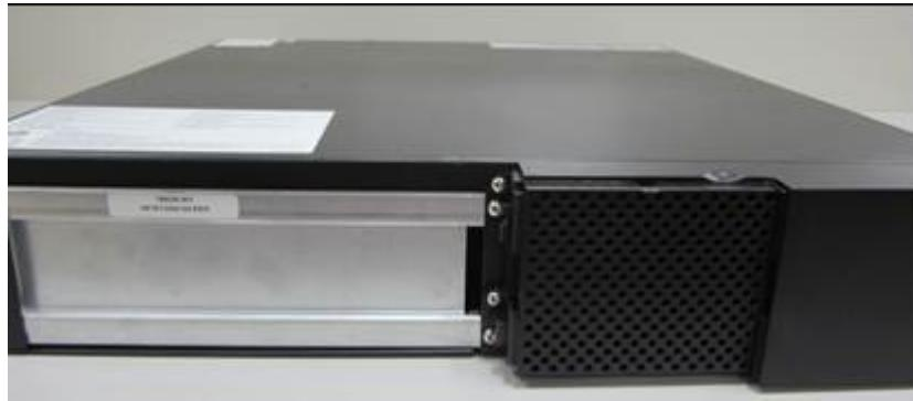
2. Loosen the screws fixing the battery door and right panel, and then remove the battery door and right panel.
