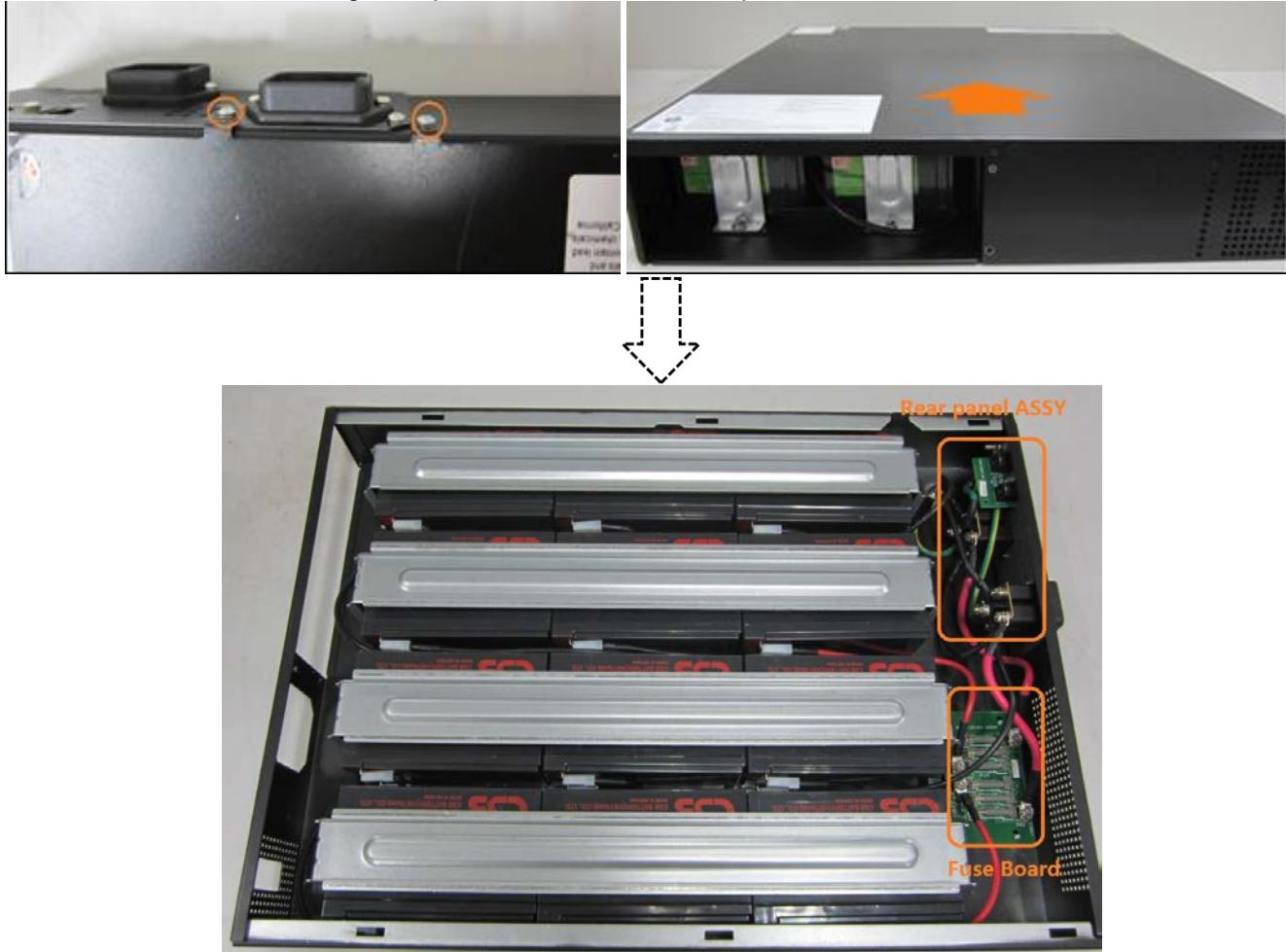
4. Disconnect the battery cables, and wrap the cable terminals with insulating tape.
