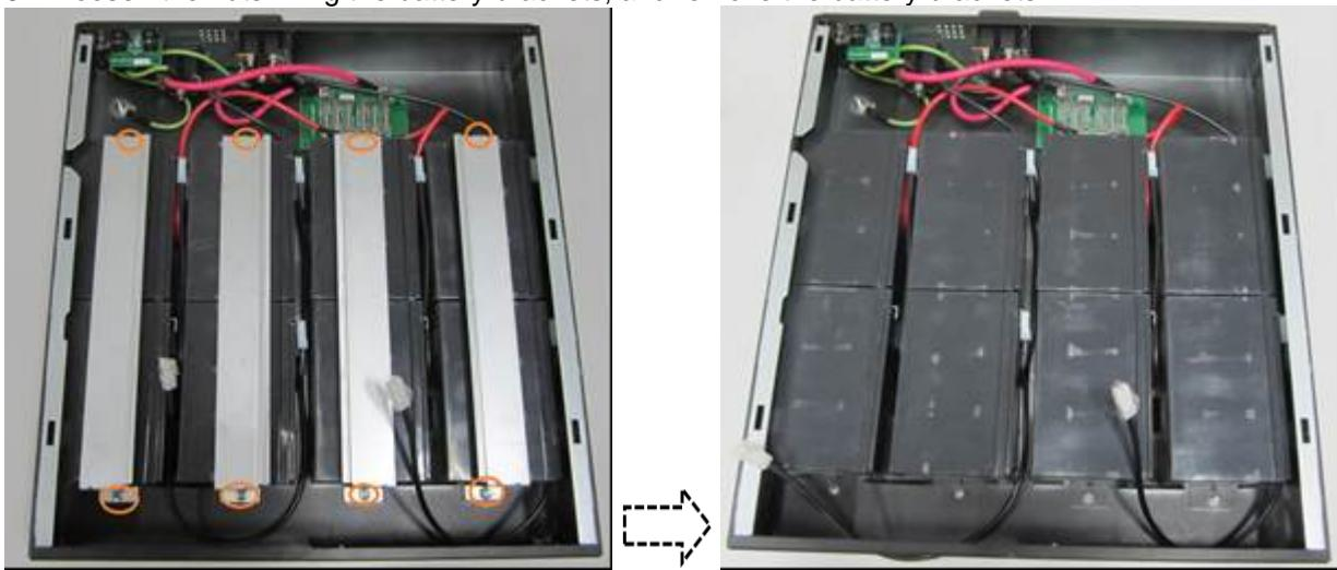
6. Stand the batteries, and disconnect the cables connecting to Fuse Board and rear panel ASSY, and then remove the batteries.
