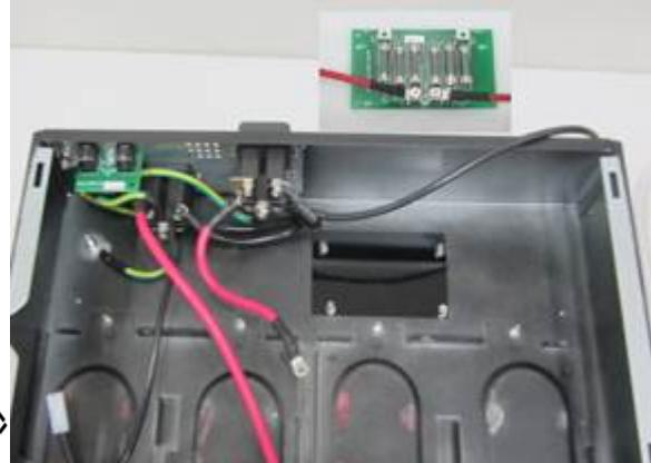
8. Loosen the nuts fixing the ground cable to the mainframe, and loosen the screws fixing the rear panel ASSY, and then remove the rear panel assembly.
