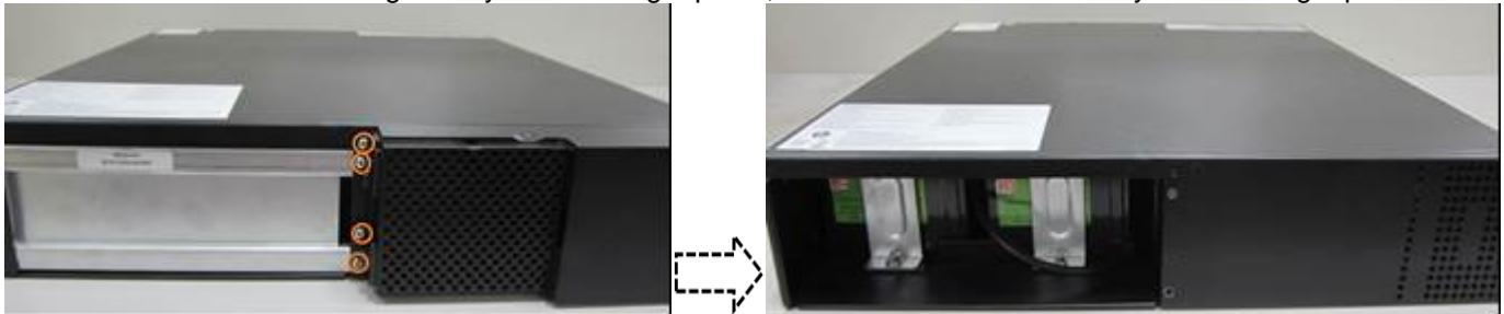
3. Loosen the screws fixing the top cover, and remove the top cover.
