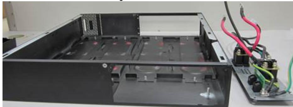
9. Disassemble the rear panel ASSY into separate parts.
