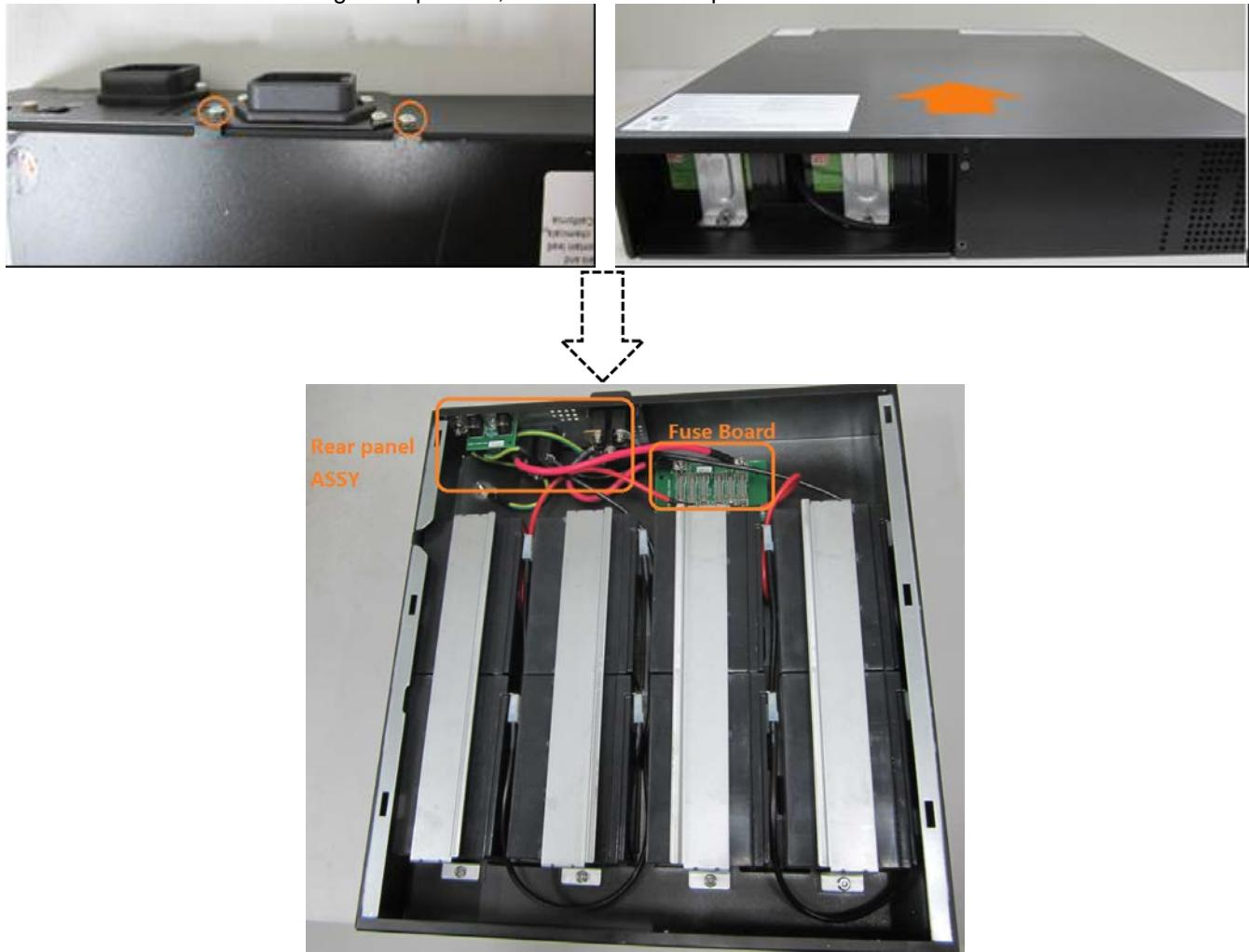
4. Disconnect the battery cables, and wrap the cable terminals with insulating tape.
