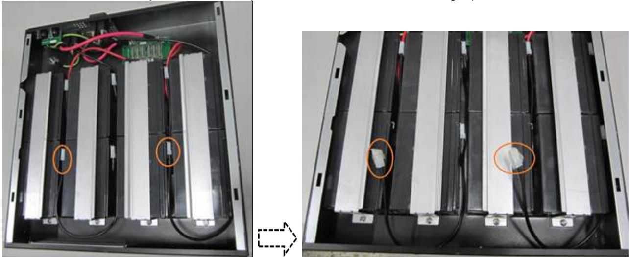
5. Loosen the nuts fixing the battery brackets, and remove the battery brackets.
