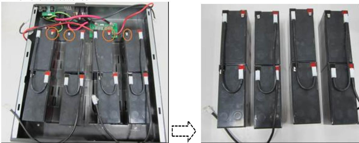
7. Loosen the screws fixing the cables on the Fuse Board, and loosen the screws fixing the Fuse Board, and then remove the Fuse Board.
