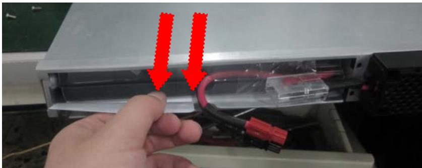
4. Loosen the screws fixing the right panel ASSY, and remove the right panel ASSY.
