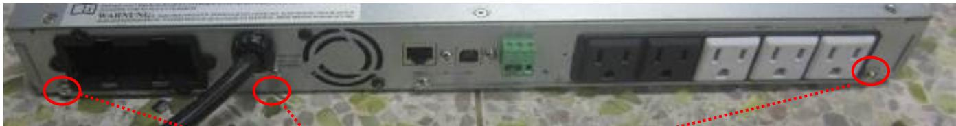
10. Remove the RPO connector, loosen the screws fixing Slot box, COM PCBA, and rear FAN, loosen the nut fixing ground cable and then remove the Slot box, COM PCBA, and rear FAN, outlet.
