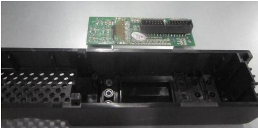
6. Loosen the screws fixing the top cover, and remove the top cover.
