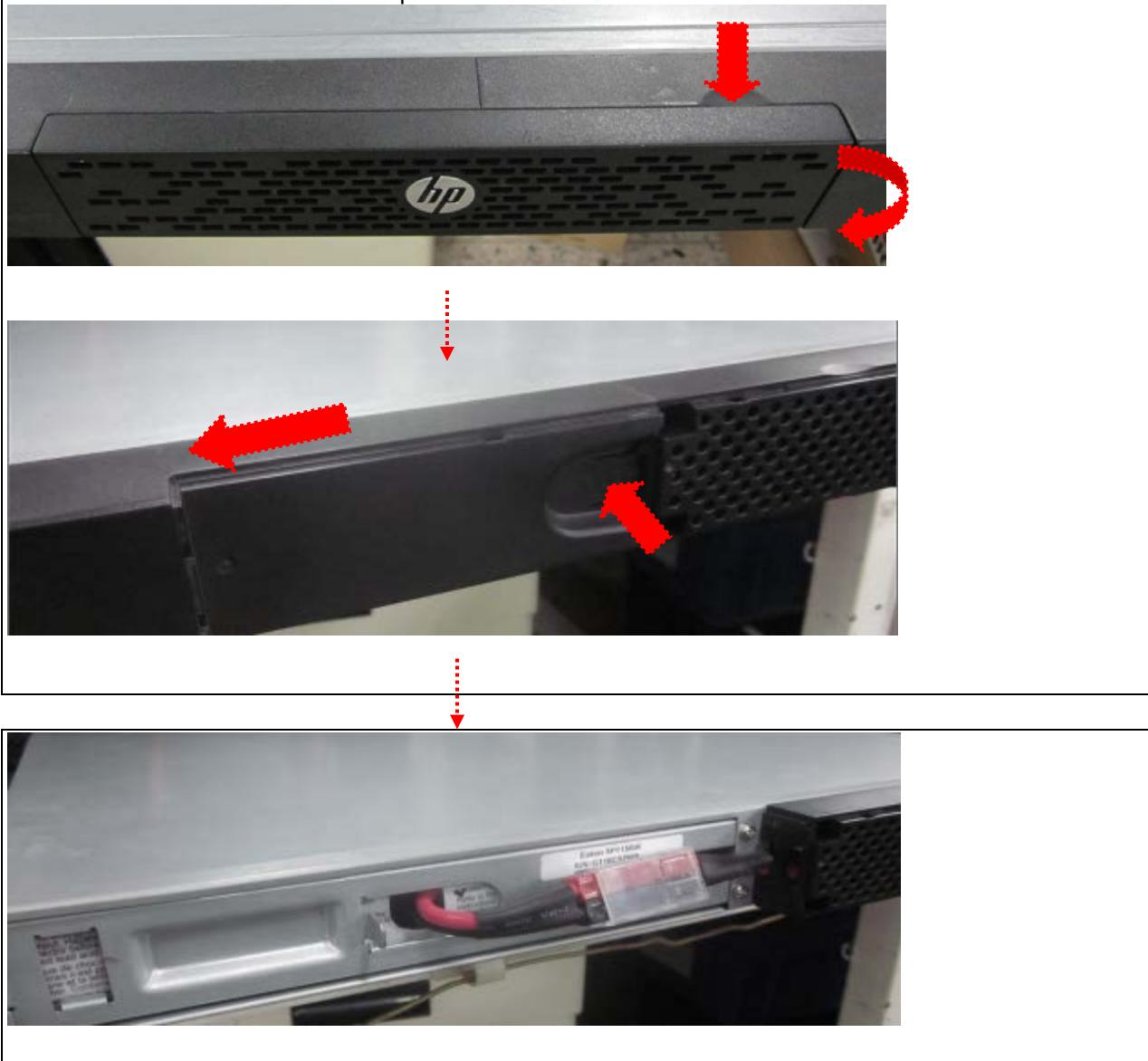
2. Disconnect the battery connector, and press on/off button to discharge the rest electricity.
