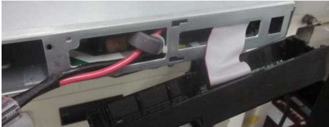
5. Disconnect the LCD cable and PCBA.
