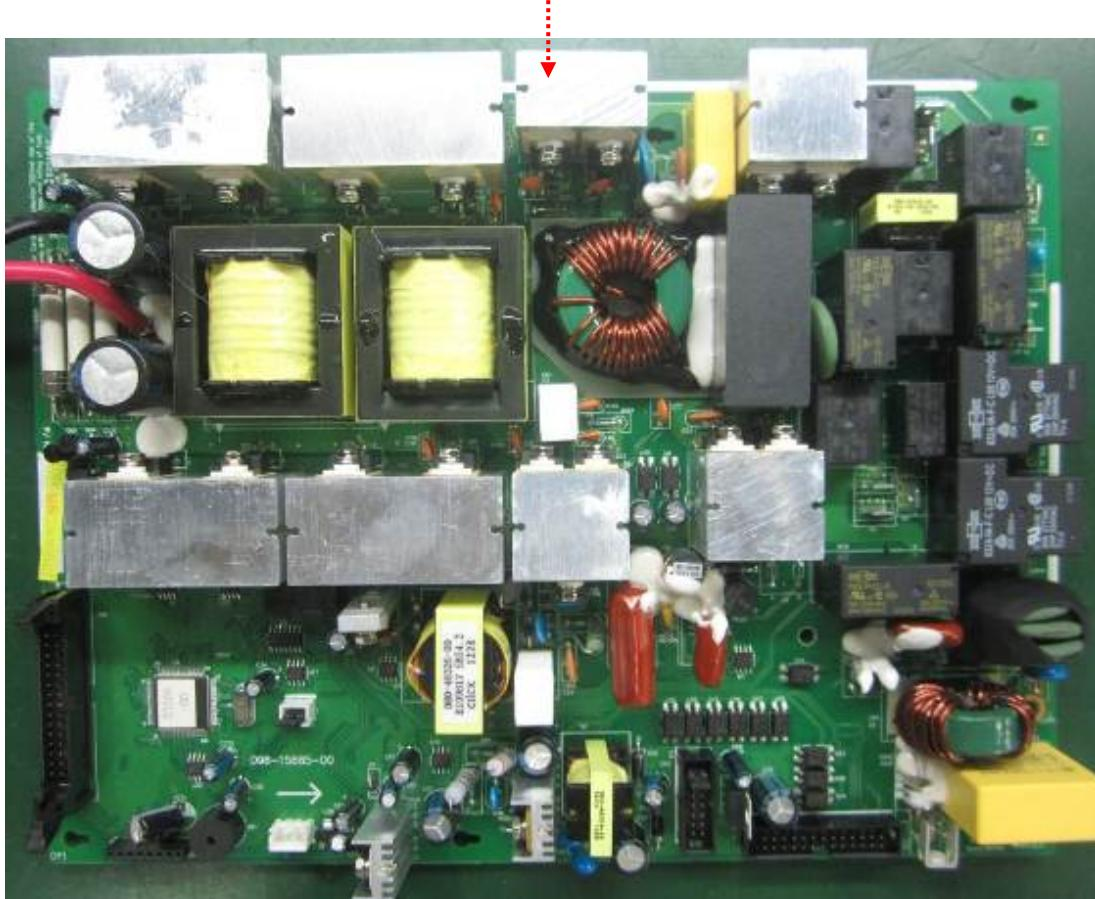
8. Cut off the cable tie, disconnect the cable connecting to COM PCBA, loosen the nuts fixing the AVR, and then remove the AVR.
