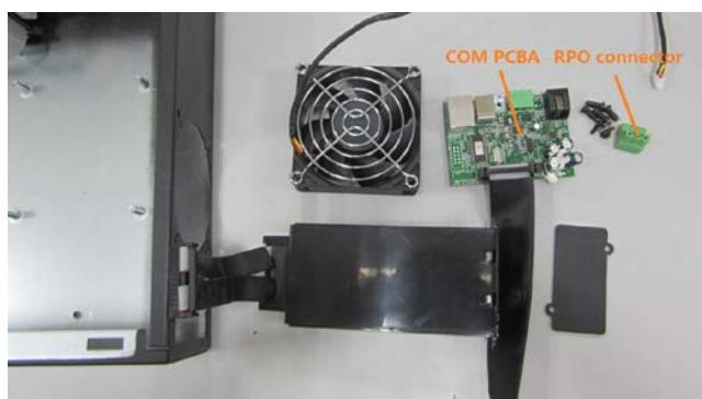
10. Disconnect the cables connecting to the I/O PCBA, loosen the nut fixing ground cable to the mainframe, loosen the screws fixing rear panel ASSY, and then remove the rear panel ASSY.
