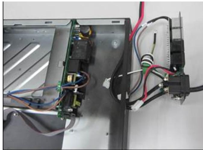
11. Loosen the screws fixing I/O PCBA, and then remove the I/O PCBA.
