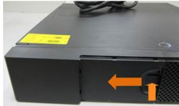
2. Disconnect the battery connector, and press on/off button to discharge the rest electricity.
