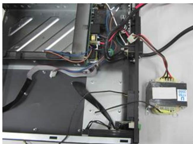
9. Remove the RPO connector, loosen the screws fixing Slot box, COM PCBA, and rear FAN, and then remove the Slot box, COM PCBA, and rear FAN.
