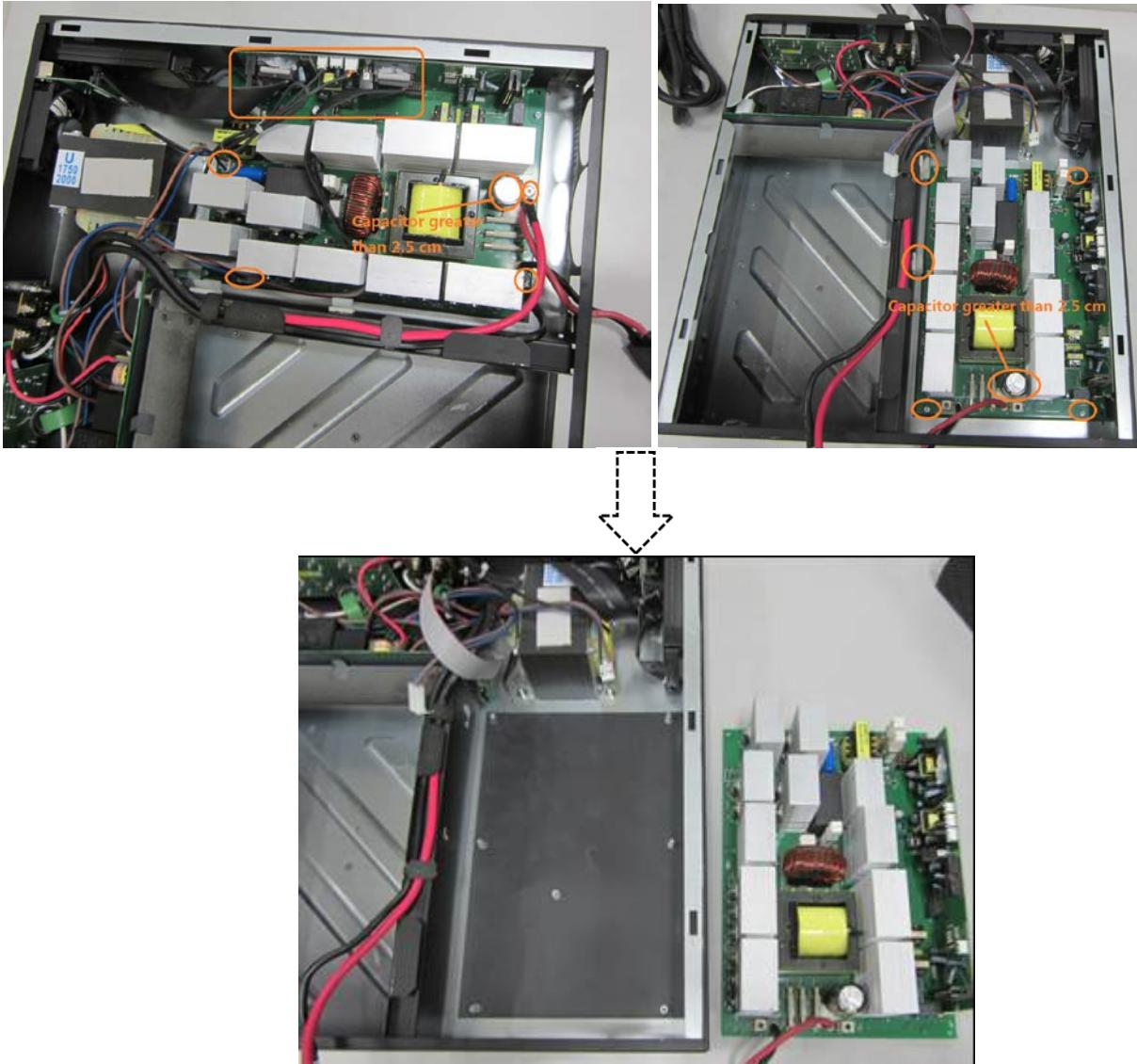
8. Cut off the cable tie, disconnect the cable connecting to I/O PCBA, loosen the nuts fixing the AVR, and then remove the AVR.
