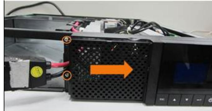
6. Loosen the screws fixing the front FAN, and remove the front FAN
