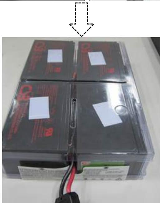
4. Loosen the screws fixing the top cover, and remove the top cover.
