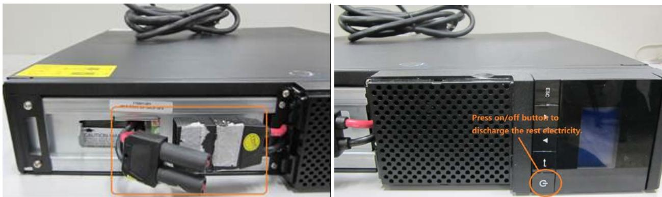
3. Loosen the screws fixing the battery door, remove the battery door, and pull out the battery.
