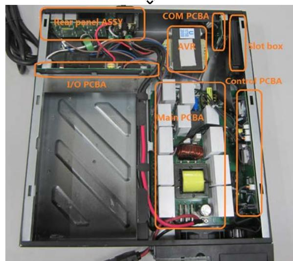
5. Disconnect the LCD cable and front FAN cable connecting to control PCBA, loosen the screws fixing the right panel ASSY, and remove the right panel ASSY
