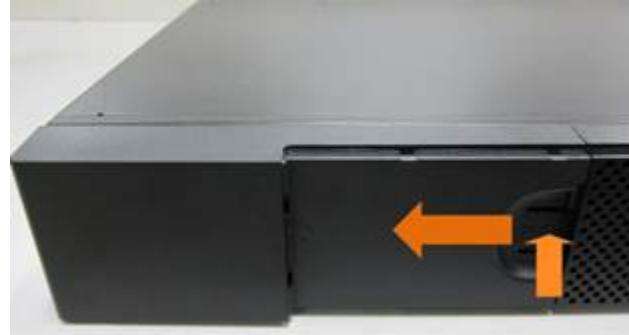
2. Disconnect the battery connector, and press on/off button to discharge the rest electricity.
