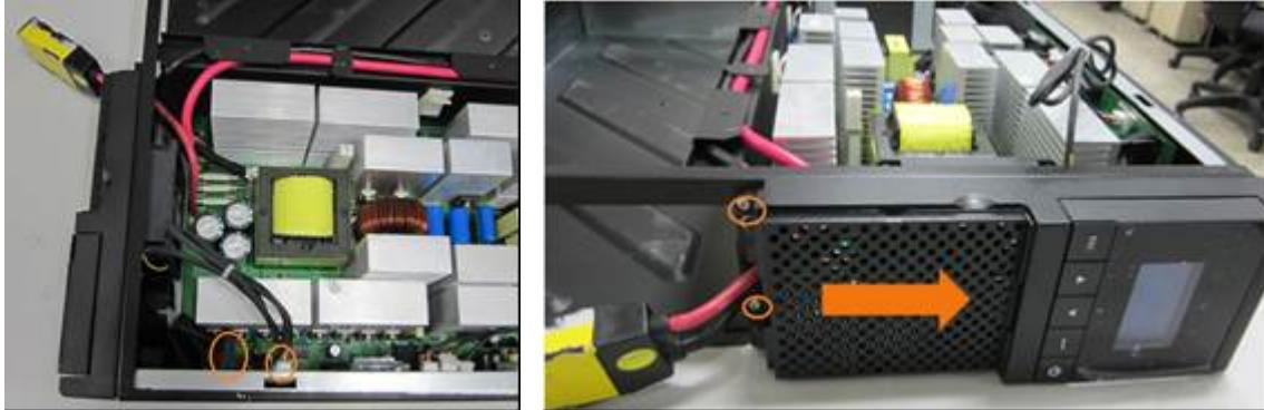
6. Loosen the screws fixing the front FAN, and remove the front FAN
