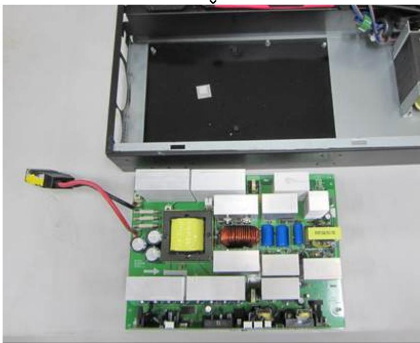
8. Loosen the screws fixing the rear panel ASSY, disconnect the cables connecting to the I/O PCBA, loosen the nut fixing the ground cable to the mainframe, and then remove the rear panel ASSY.
