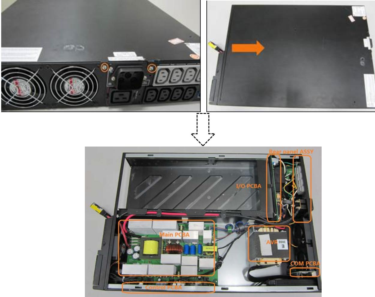
5. Disconnect the LCD cable and front FAN cable connecting to control PCBA, loosen the screws fixing the right panel ASSY, and remove the right panel ASSY
