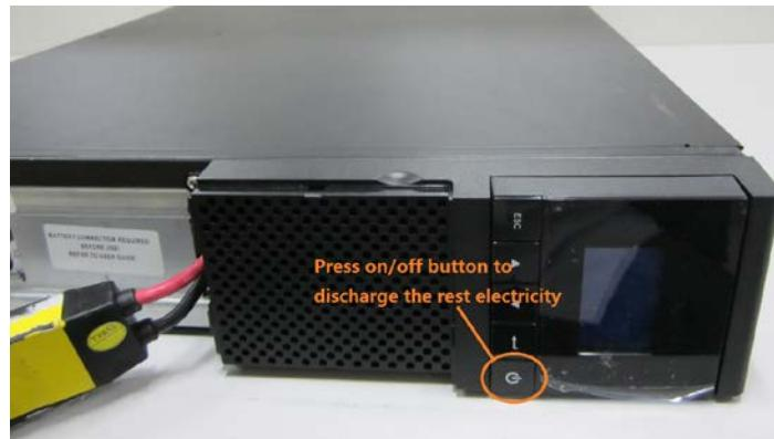
3. Loosen the screws fixing the battery door, remove the battery door, and pull out the battery.
