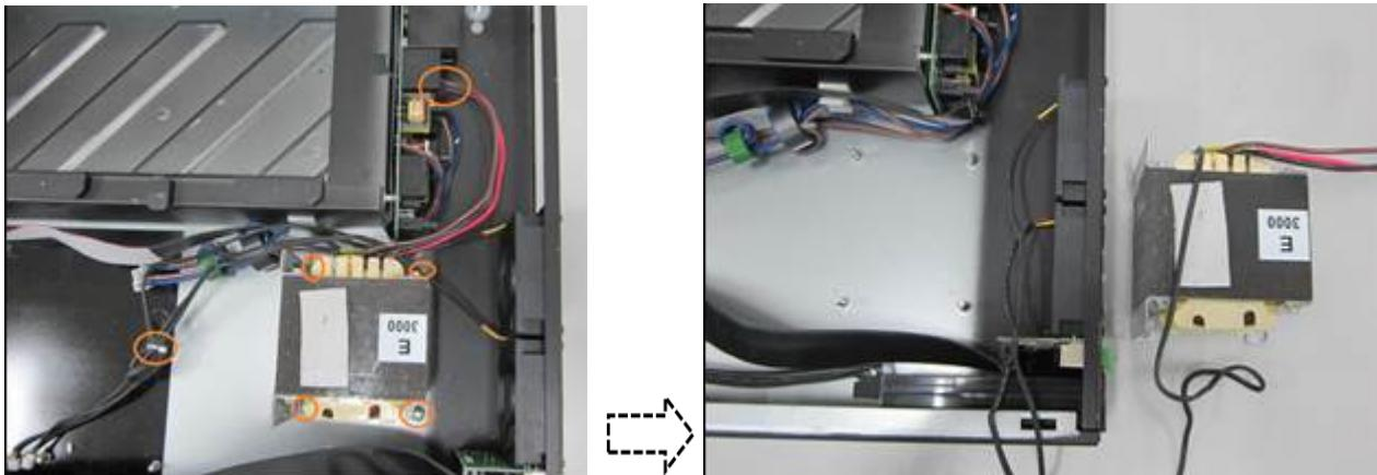
10. Remove the RPO connector, loosen the screws fixing Slot box, COM PCBA, rear FANs, and remove Slot box, COM PCBA, and rear FANs.
