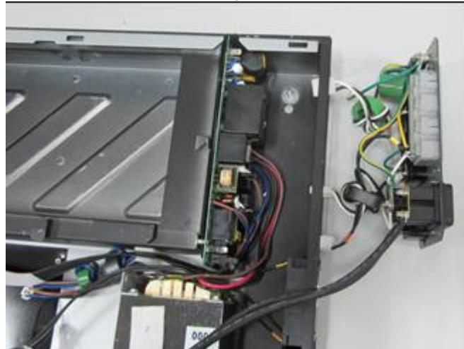
9. Cut off the cable tie, disconnect the cables connecting to I/O PCBA, loosen the nuts fixing the AVR, and then remove the AVR.
