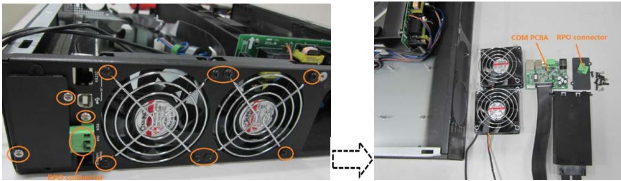
11. Loosen the screws fixing I/O PCBA, and then remove the I/O PCBA.
