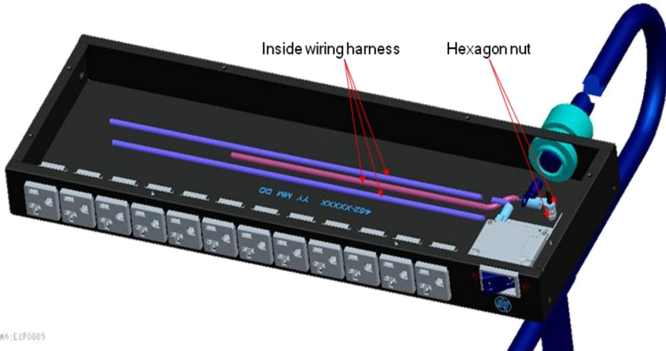
4. If needed, remove cable and cable gland
