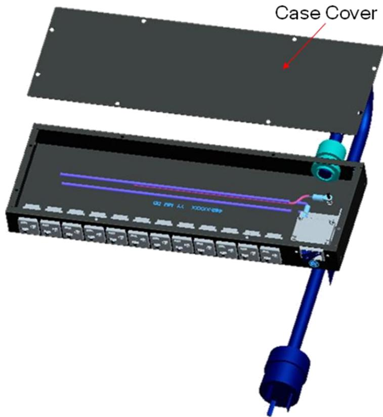
3. Remove hexagon nut and pull-out all the inside wiring harnesses
