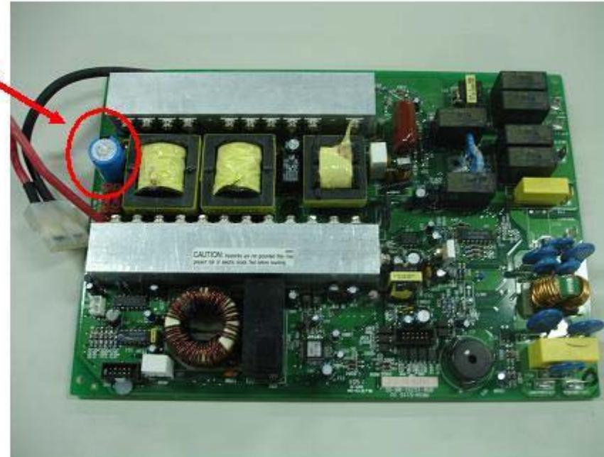
The PSDR PCB assembly of Low Voltage (US/TWN/JPN) unit
