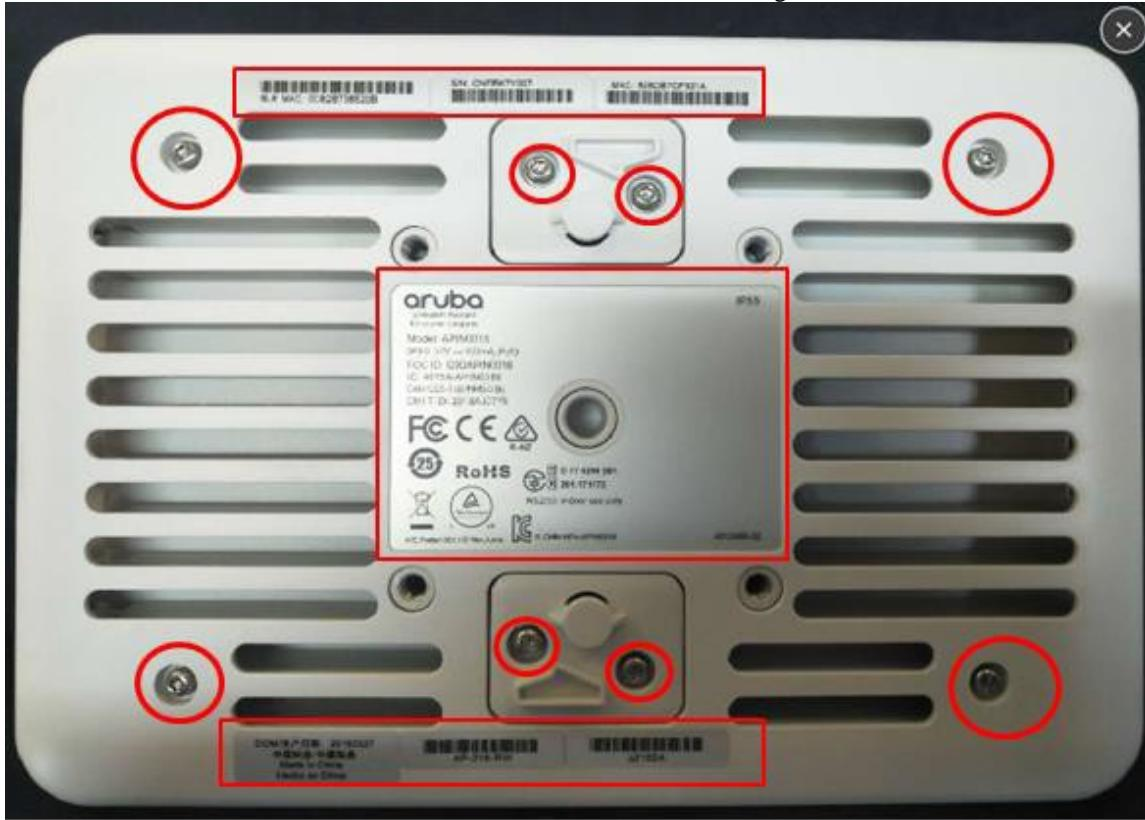
2. Use T20 screw drive to remove 6pcs screws on Bottom Cover
