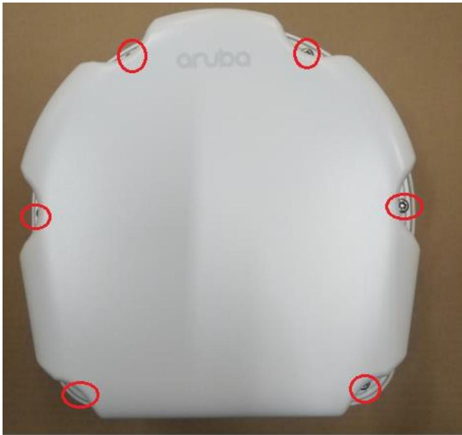
3. Use Cross-head screwdriver to remove 4 screws on the antenna cover
