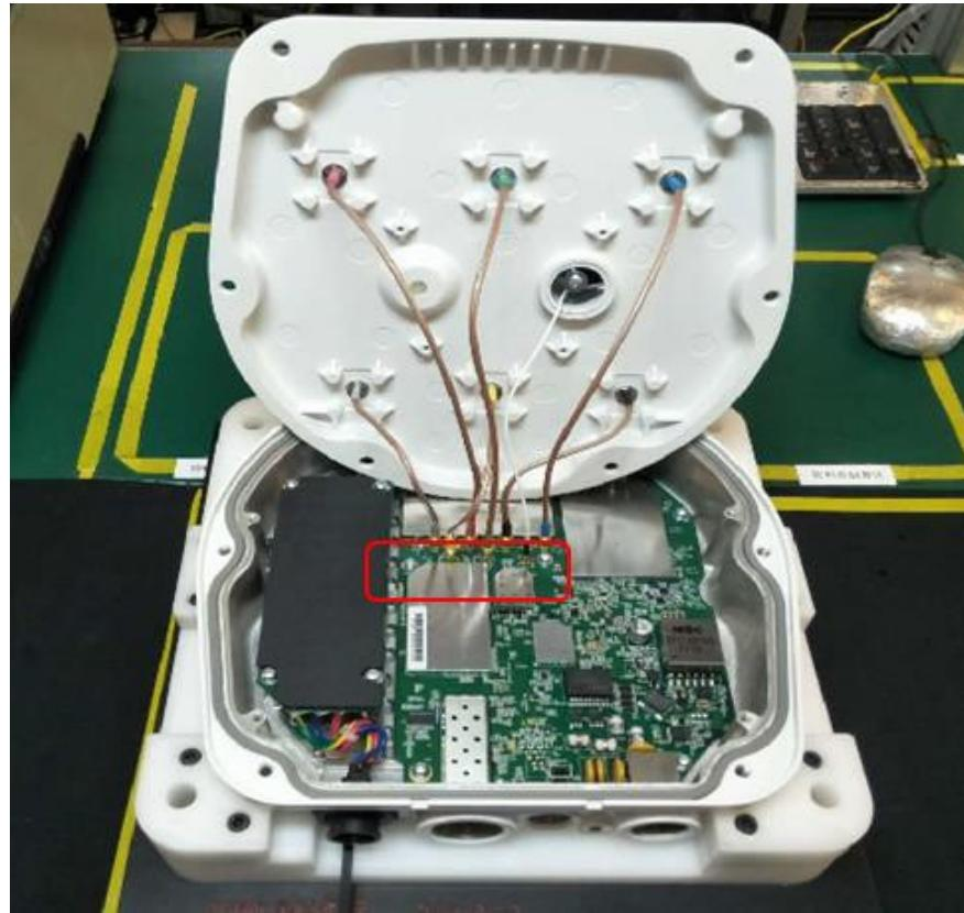
5. Use Cross-head screwdriver to remove screws on the PCBA and AC Module.
