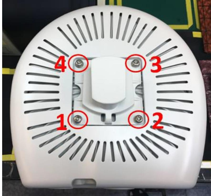
2. Use Cross-head screwdriver to remove screw on the TOP
