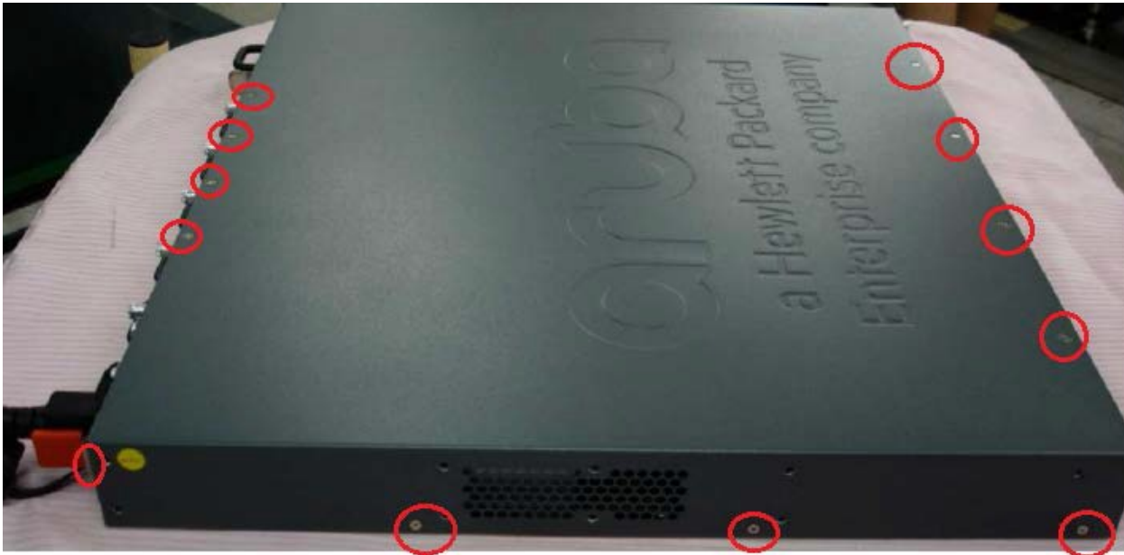
Figure 1 : Remove all screw on chassis, total 16pcs.
