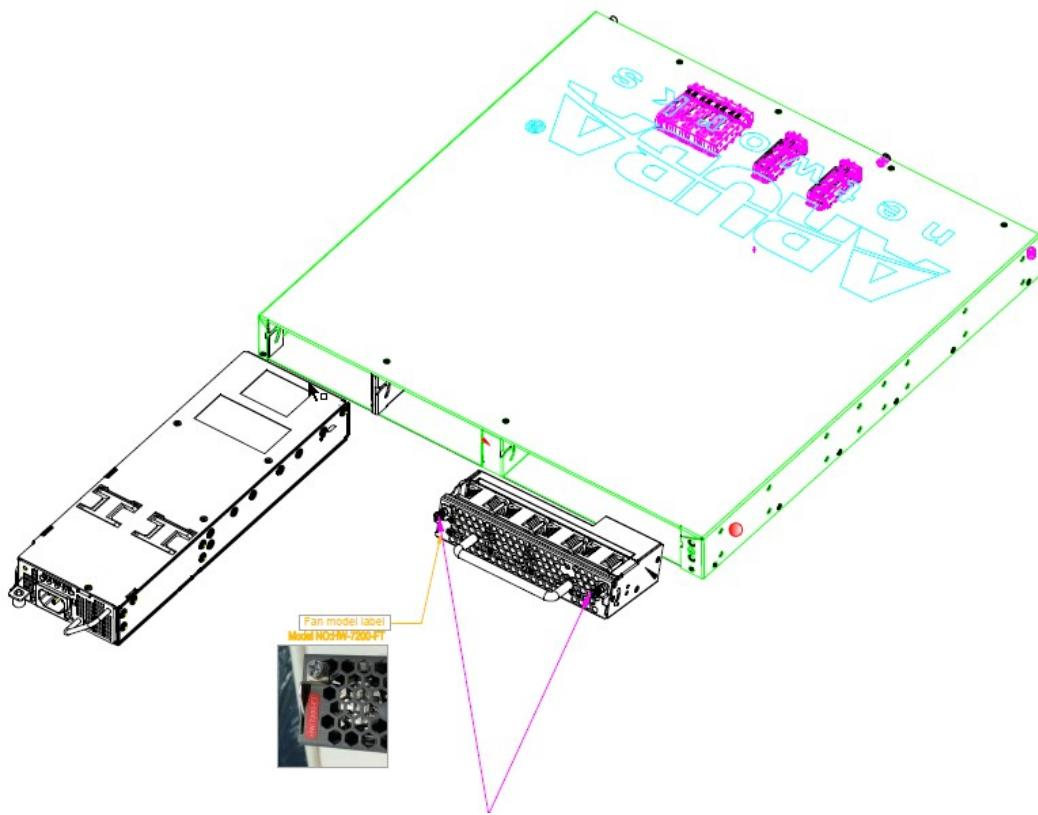
3. Open the chassis by removing the screws on the top cover.
