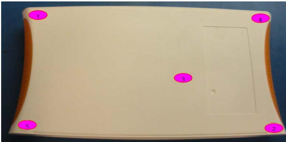
2. Uninstall the CPU board by removing 4 screws.
