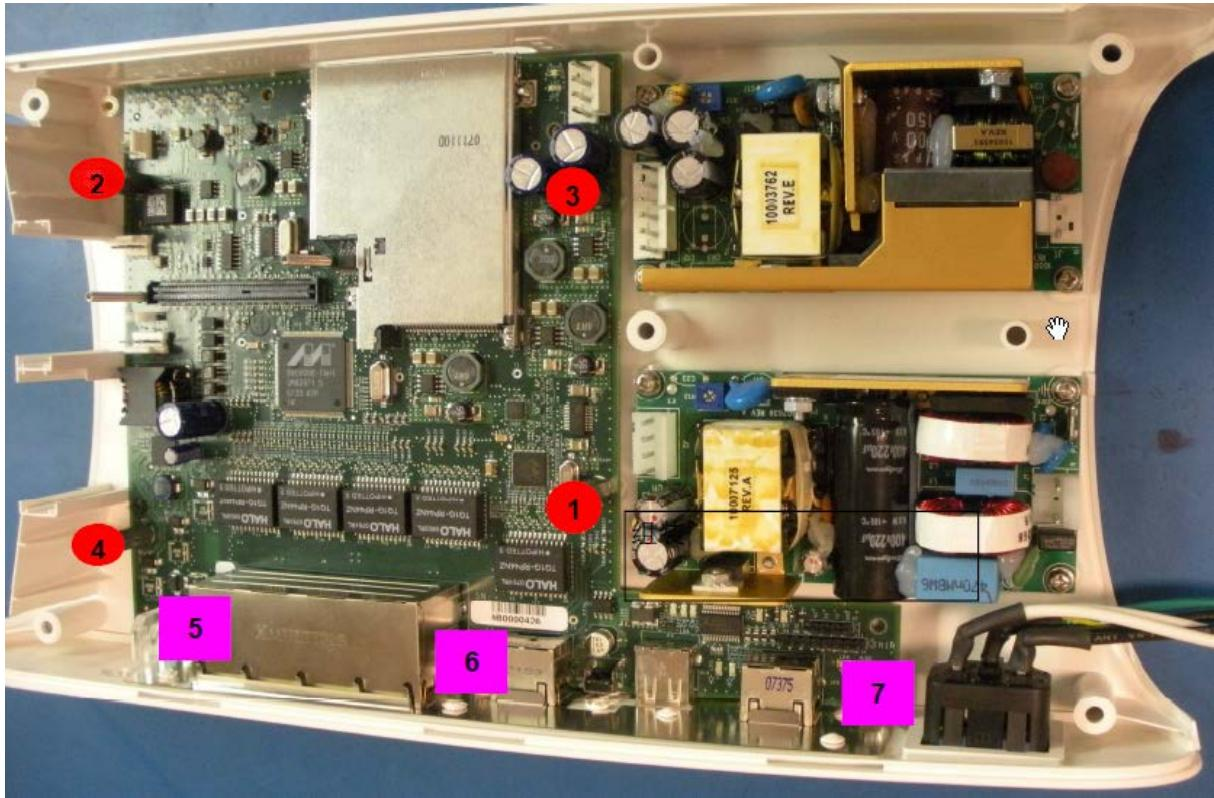
6. Uninstall the main board by removing the 4 screws (1,2,3,4).
